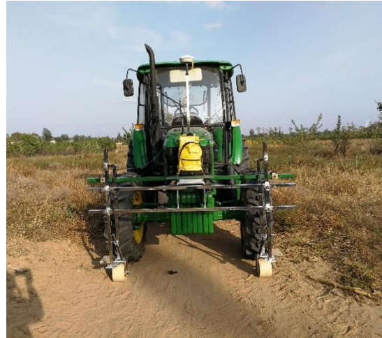
Fig. 2 - Terrain profile and tractor vibration test on field road
