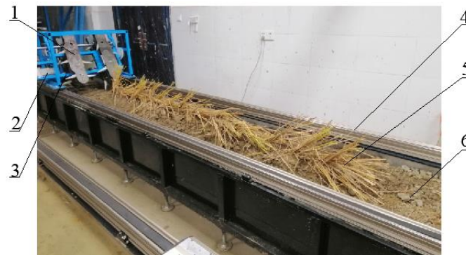
Fig. 6 - Performance test rack of double-layer chain finger grain lifter
