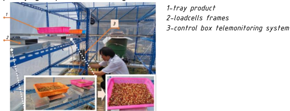
Fig. 3 – Telemonitoring devices integrated into the solar dryer
