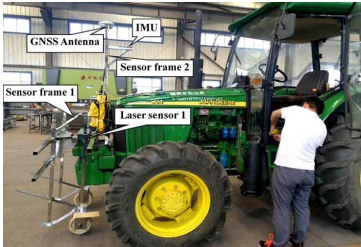
Fig. 1 - Profiling apparatus mounted on the front counterweight of a tractor
