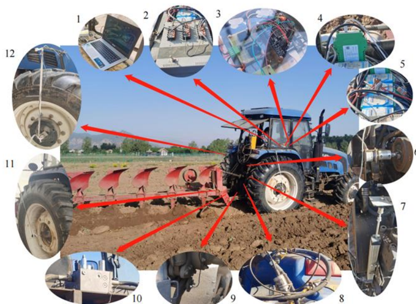
Fig. 5 – Field test platform of tractor electro-hydraulic hitch control system
