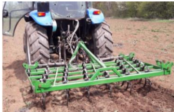
Fig. 3 – The 2 m working width version of the MCLS with an 80 HP tractor
