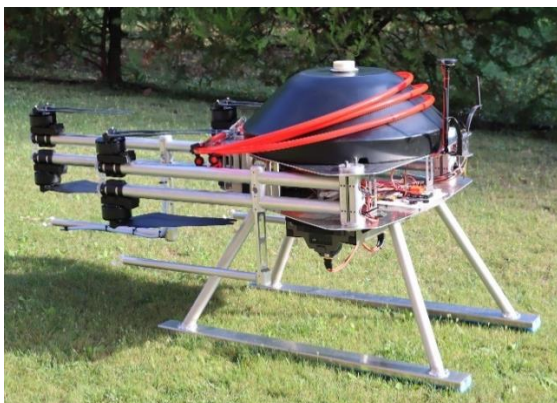
a) Functional model - folded for transport
