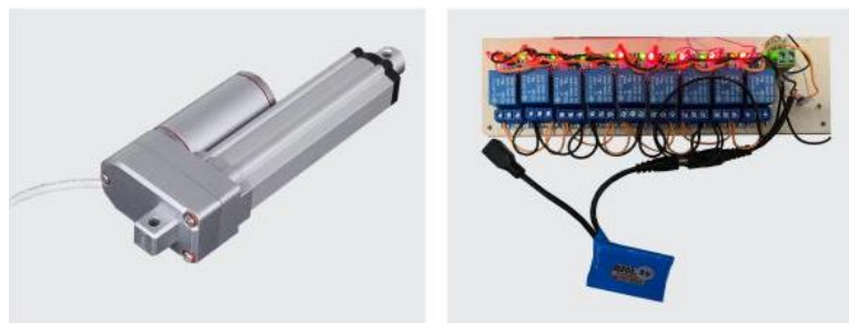
(a) Electric push rod (b) Relay modules Fig. 6 - Electric push rod and relay modules
