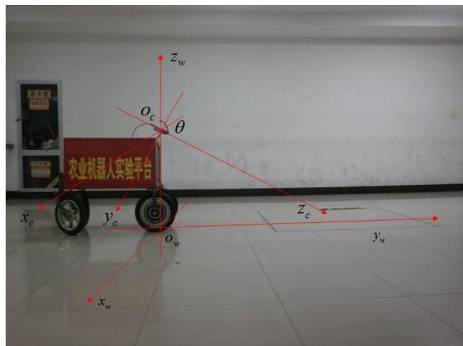
Fig. 1 - The overall structure of the agricultural robot experimental platform
