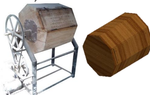
Fig. 8 - Handmade tagua polishing machine with its virtual drum model
