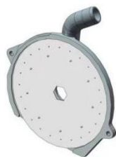
Fig. 3 – Structure of seed plate and vacuum chamber
