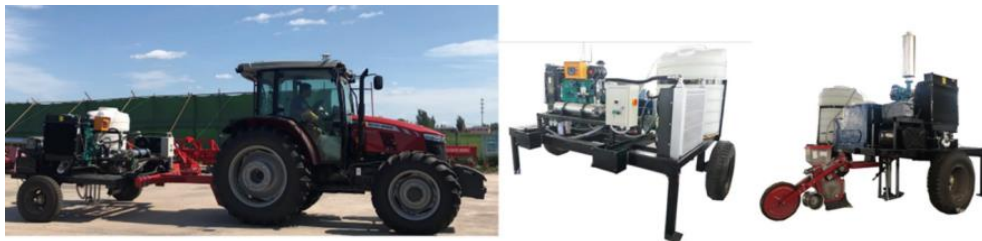
Fig. 5 - Non-contact jet cutting stalk-free tillage anti-blocking device (Hu et al., 2020)
