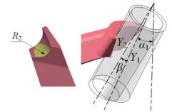
Fig. 5 - Schematic diagram of the improved spoon hole
