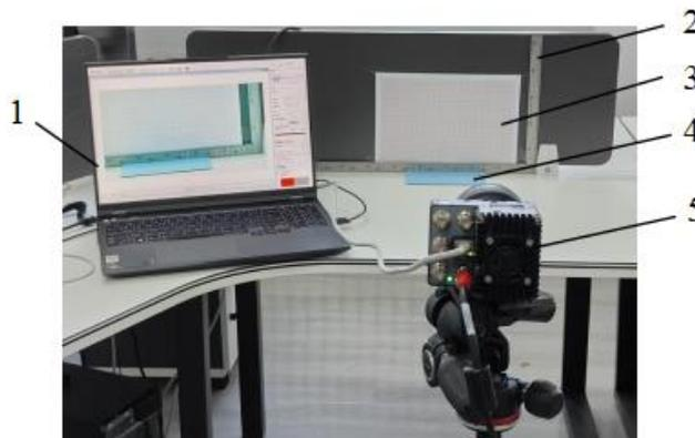
Fig. 6 - Collision restitution coefficient measurement test
