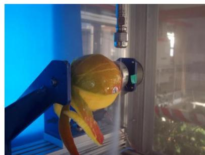
(b) Cut of a mango cortex controlled by photography
