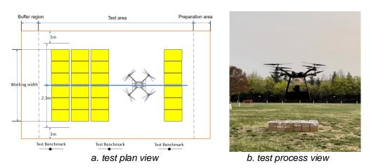
Fig. 11 - UAV seeding performance test
