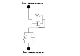
Fig. 6 – Schematic of soil particle contact modeling
