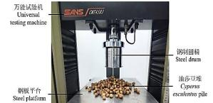
Fig. 4 – Physical Repose angle test of Tiger nut tubers
