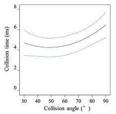
Fig. 10 - Influence of collision angle on collision time
