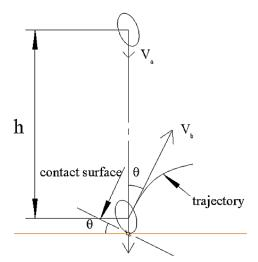
Fig. 8 - The schematic diagram of the seed collision motion
