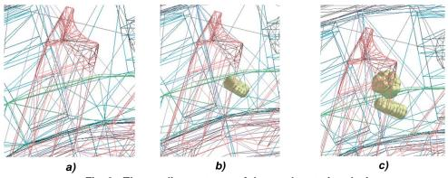
**Fig. 9 - The seeding statuses of the seed-metering device** a) Leakage sowing state; b) Qualified sowing state; c) Multiple sowing state
