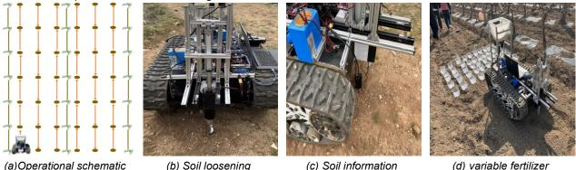
al schematic (b) Soil loosening (c) Soil information (d) variable fertilizer collection application
