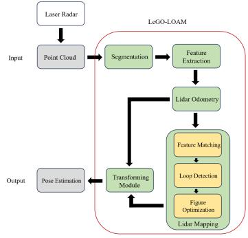
Fig. 1 – LeGO-LOAM algorithm flow
