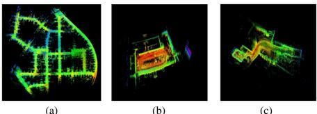
Fig. 8 – Maps constructed by the improved LeGo-LOAM algorithm
