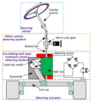
Fig. 2 - Schematic diagram of E-HCSS
