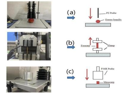
Fig. 1 - (a) Puncture test of Cerasus humilis; (b) Tensile test of exocarp; (c) Compression test of mesocarp
