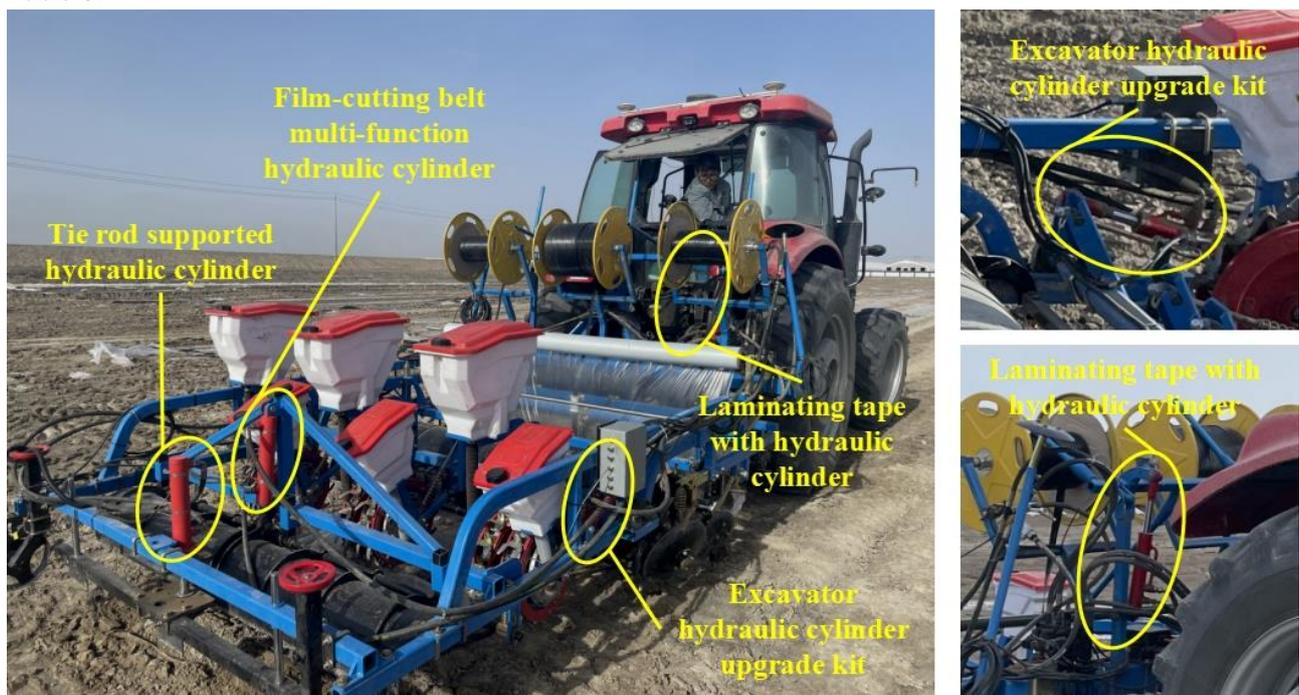
Fig. 7 - Installation diagram of hydraulic cylinder
