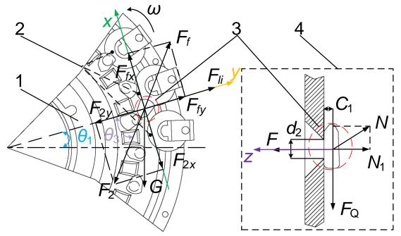
Fig. 4 - Schematic diagram of the forces on the excess seeds after entering the clearing area 1. seeding plate; 2. seed scraper; 3. excess seed; 4. forces of excess seed z-axis direction.
