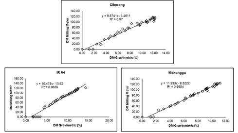
Fig. 4 - Relationship of milling degree analyzed by Gravimetric method and measured by milling meter
