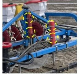
Fig. 4 - Installation diagram of Hydraulic limit sensor
