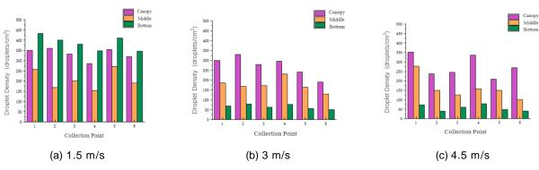
Fig. 11 - Distribution of droplet deposition characteristics at each sampling point for different flight speeds
