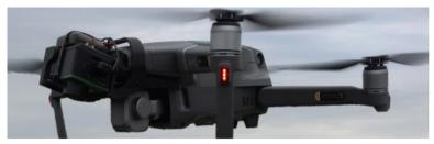
Fig. 2 - DJI Mavic 2 Pro with MAPIR Survey3W camera mounted
