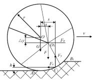
Fig. 8 - Force diagram of profiling wheel
