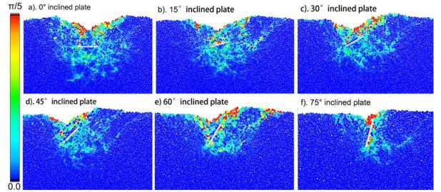
Fig. 7 – Plates with various inclination angles penetrated into the soil at a depth of 100 mm
