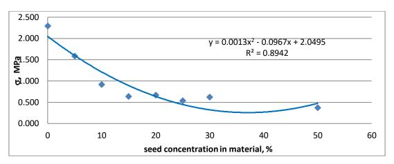
Fig. 3 - Variation of the crushing limit resistance of the sludge matrix composite material and seed husk insert, with the concentration of seed husks
