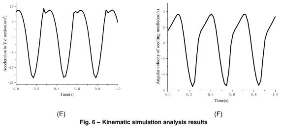
A-Displacement diagram of F point of the tip of seedling needle; B-Variation of horizontal velocity of rice interpolation mechanism; C-Variation of vertical velocity of rice interpolation mechanism; D-Accelerating change of horizontal velocity of rice transplanting mechanism; E-Accelerating change of vertical direction of rice transplanting mechanism; F-Angular velocity change rule diagram of rice-planting mechanism.
