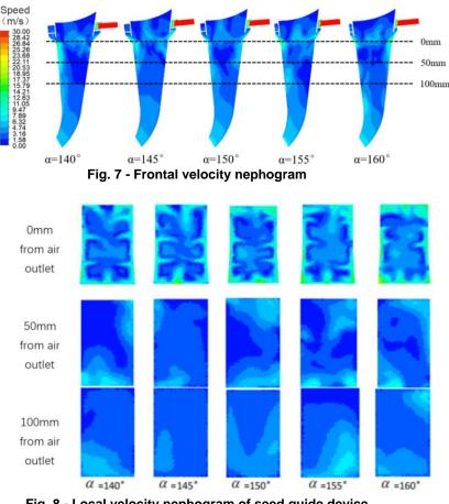
Fig. 8 - Local velocity nephogram of seed guide device
