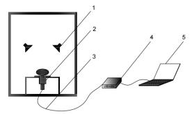
**Fig. 2 - Structure of transmission spectrum data acquisition system** 1 - Halogen lamp; 2 – Collimator; 3 - Fiber optic; 4 - USB4000 Spectrometer; 5 - Laptop
