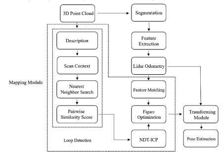
Fig. 3 – System architecture diagram of the improved algorithm in this paper
