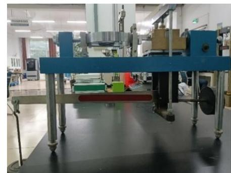
Fig. 3 – ZJ type strain control type straight shear instrument
