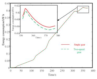
Fig. 8 - Comparison in one transportation test cycle
