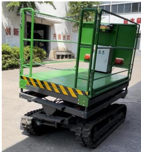
**Fig. 13 - Working platform prototype**
