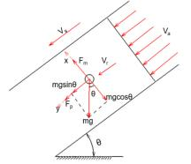
**Fig. 3 - Schematic diagram of seed force in the seed guide device** Note: mg - Gravity;  $F_m$  - Magnus effect force;  $\theta$  - air flow angle;  $v_r$  - relative velocity of seed and air flow;  $v_a$  - air velocity;  $v_s$  -seed velocity
