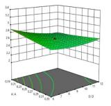
(a) Effect of AC on soil accumulation angle
