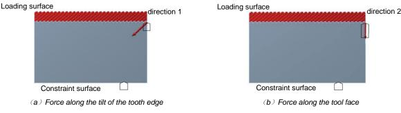
Fig. 10 - Diagram of constraints and loads
