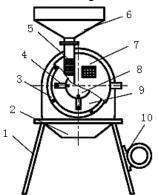
**Fig. 1 - Structure diagram of the hammer mill** 1-Frame; 2-Outlet; 3-Sieve frame and sieve; 4- Hammer; 5-Air inlet of feeding mouth; 6-Feeding hopper; 7-Cover plate of grinding chamber; 8. Hammer frame; 9-Grinding chamber; 10-Motor
