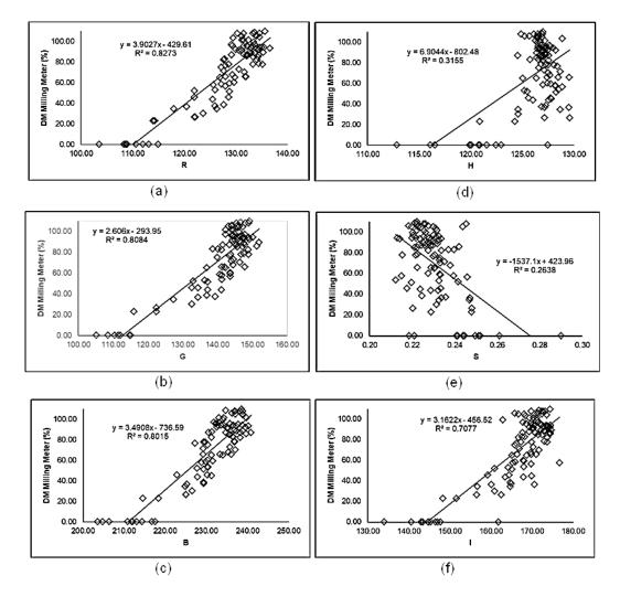
Fig. 6 - Correlation between the degree of milling measured by milling meter and estimated using fluorescence image on Ciherang variety using (a) red signal, (b) green signal, (c) blue signal, (d) hue color component, (e) saturation color component, and (f) intensity color component
