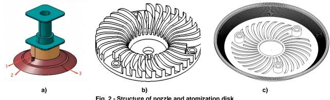
Fig. 2 - Structure of nozzle and atomization disk 1. brushless motor; 2. Inlet; 3. fogging tray
