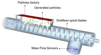
Fig. 4 - Simulation Model of Shaftless Screw
