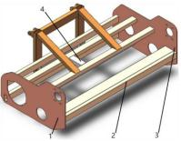
**Fig. 1 - Simplified frame for pickup header** 1.Right side panel of the frame; 2. Frame front beam; 3.Left side panel of the frame; 4. Frame rear beam.
