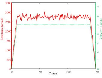
Fig. 2 - Test cycle of rotary tillage
