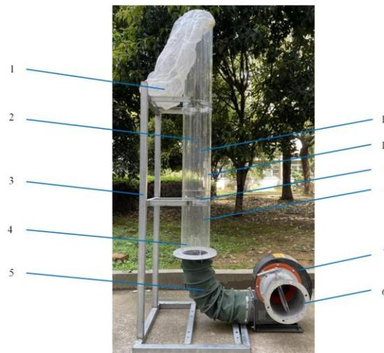
**Fig. 1 - Suspension speed experiment device**
