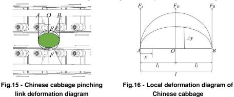
It can be seen from Figure 15 that the extrusion force of Chinese cabbage at point O, the force of point A and point B are  $F_A$  and  $F_B$  respectively:
