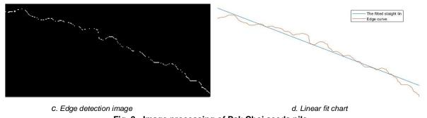
Fig. 8 - Image processing of Pak Choi seeds pile
