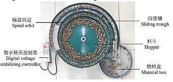
Fig. 10 – Electromagnetic vibration hopper test
