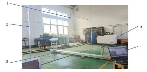
Fig. 7 - Test system for centrifugal nozzle parameters
