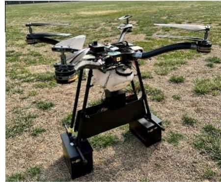
Fig. 2 - Physical drawing of rice flying seeding drone
