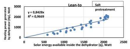
Fig. 10 – Heating energy generated by the lean-to solar dehydrator against solar energy inside the dehydrator for salt pretreatment
