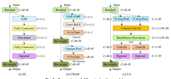
**Fig. 3 - Comparison of different attention modules** *C, H, W – the number of channels, height, and width of the feature map; GAP – Global Avg Pool; GMP – Global Max Pool;*
