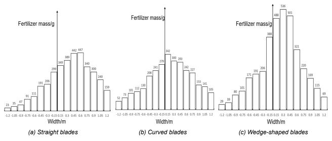
Fig. 9 - Histogram of fertilizer spreading distribution
