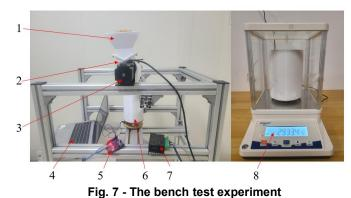
1 – seed box; 2 – seed dispenser with external groove wheel; 3 – stepper motor; 4 – computer; 5 – Arduino board;
