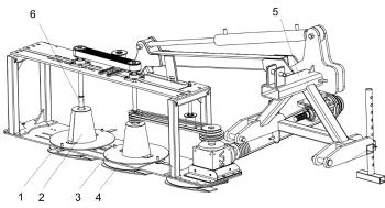
Fig. 5 - Structure diagram of cutting test bench
