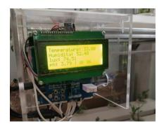
Fig. 14 – Controller board
