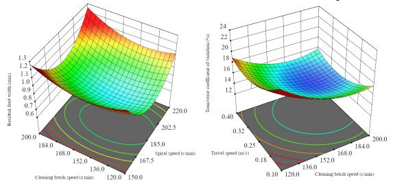
Fig. 10 - Response surface for the interaction between residual feed width and transverse coefficient of variation (a) x<sub>3</sub>=0.4 m/s (b) x<sub>1</sub>=185 r/min
