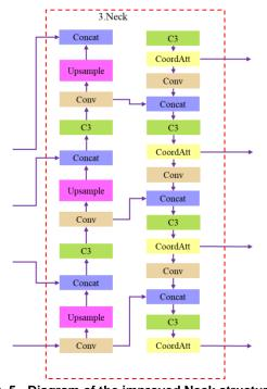
Fig. 5 - Diagram of the improved Neck structure
