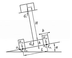
(a) The platform is longitudinal to the slope
