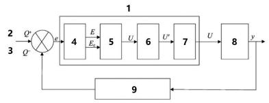
Fig. 8 – Schematic Diagram of the Header Height Fuzzy Control Principle (Zhou et al., 2019)
