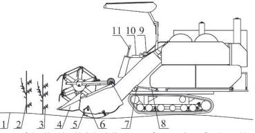
Fig. 4 - Schematic Diagram of the Header-Height Adjustment System for a Soybean Harvester (*Ni et al., 2021*) 1. Ground; 2. Soybean plant; 3. Bottom pod of soybean; 4. Header; 5. Profiling mechanism; 6. Angular transducer; 7. Articulated mechanism; 8. Double-acting hydraulic cylinder; 9. Controller; 10. Solenoid directional valve; 11. IPC.
