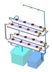
Fig. 3 – Water supply and misting system
