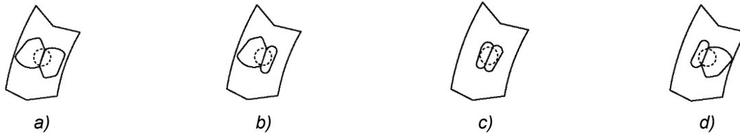
Fig. 2 - Different states of compression attachment of two seeds on shape hole
