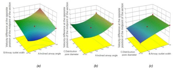
Fig. 16 - Influence of various factors on the velocity difference of the opposite position of the midpoint of the section
