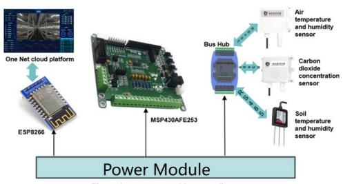
Fig. 4 - Lot system architecture diagram
