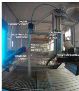
(a) Experiment setup of water-jet automation
