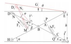
Fig. 2 - Schematic diagram of lifting and longitudinal leveling structure
