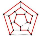
Fig. 1 - Hamiltonian circuit schematic diagram
