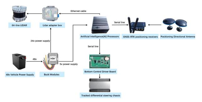
Fig. 5 – Hardware Connection Diagram of Orchard Work Robot
