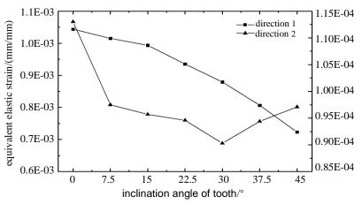
Fig. 15 - Rule of equivalent elastic strain of blade with inclination angle of tooth
