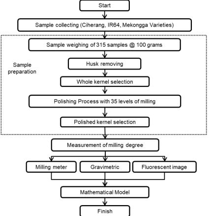
Fig. 1 - The development of a mathematical model for rice milling degree estimation using fluorescent images
