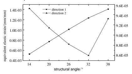
Fig. 18 -Rule of equivalent elastic strain of blade with structural angle
