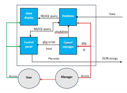
Fig. 8 – Web server programming module block diagram
