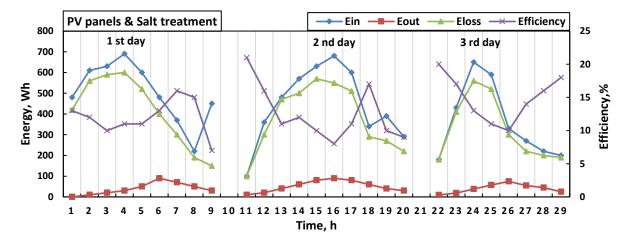
Fig. 12 – The calculated energy input (E<sub>in</sub>), energy output (E<sub>out</sub>), energy loss (E<sub>loss</sub>), and efficiency for collector, dryer, and PV for salt treatment of slices and halves tomatoes
