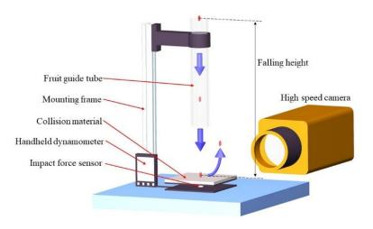
Fig. 3 - Schematic diagram of the fruit drop test
