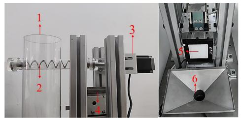
Fig. 7 - Bench Trial 1- Inlet; 2- Sampling Screw; 3- Drive Motor; 4- Vibrating Feeder and its Chute; 5- Backlight; 6- Receiving Hopper
