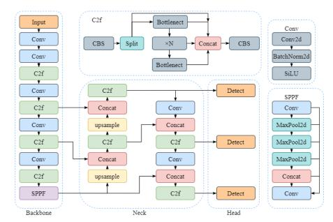
Fig. 1 - YOLOv8n network structure diagram
