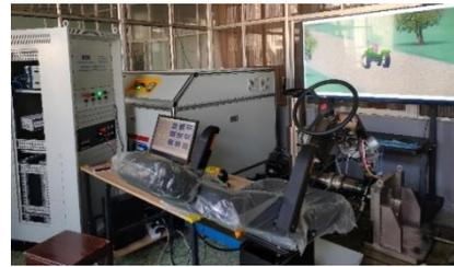
Fig. 5 - Tractor HIL steering test bench
