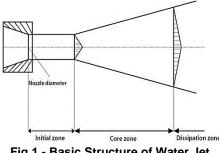
Fig.1 - Basic Structure of Water Jet
