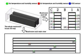
Fig. 5 - Three-dimensional map of sensor layout position
