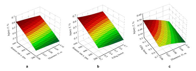
Fig. 5 - Response surface of the magnitude of the maize grain damage depending on: a) T = f(D; n); b)  $T = f(n; \psi);$  c)  $T = f(\psi; n)$
