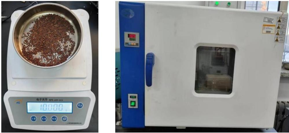
Fig. 3 - Moisture content testing device
