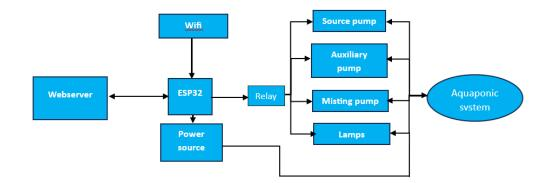
Fig. 7. Control and peripheral module's block diagram
