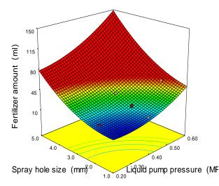
Fig. 6 - Response surface diagram of the influence of spray hole diameter and liquid pump pressure on fertilizer application rate
