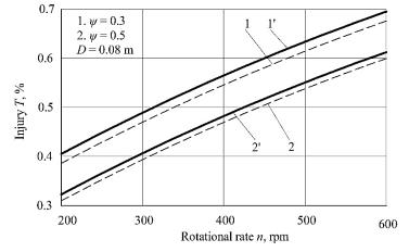
Fig. 7 - Dependences of damage to the grain material T, %, caused by the screw working body (a solid line)
