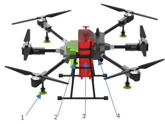
Fig. 1 - Schematic diagram of centrifugal plant protection drone structure 1. centrifugal nozzle; 2. plant protection drone; 3. medicine cabinet; 4. control box
