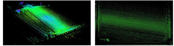
Fig. 17 – High-precision 3D point cloud map of the vineyard
