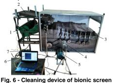
*1* - fan; 2 - oscillation grain pan; 3 - bionic screen; 4 - high-speed camera; 5 - motor; 6 - computer; 7 - frequency converter.
