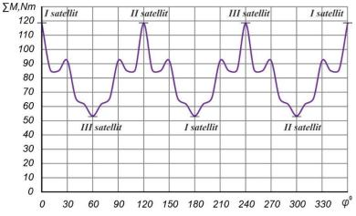
Fig. 4 – Changing graph of total resistance moment affecting the rotor's shaft of the rotary tiller with three satellite tillers located at 120<sup>0</sup>
