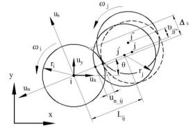
Fig. 2 – The position (displacement) changes in the normal and tangential directions
