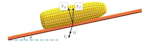
Fig. 5 - Front view of the cob and the leftward circular tube type concave plate under force
