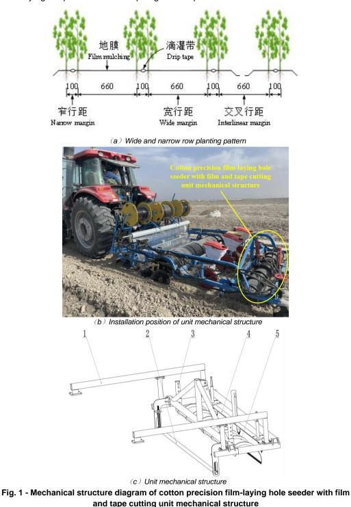
1. Frame 2. Limit rods 3. Adjustable height mechanism for the curved blade 4. Fixed strap assembly 5. Curved ripper blade
