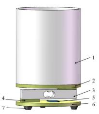
**Fig. 2 - The schematic diagram of the weighing unit structure** 1 – weighing cylinder; 2 – upper fixed plate; 3 – strain gauge pressure sensor; 4 – spacer; 5 – HX711 converter chip; 6 – lower fixed plate; 7 – foot pad
