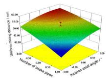
c) Effect of the number of air inlet pipes and the axial angle of the incision on the uniform mixing distance
