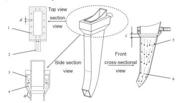
**Fig. 2 - Overall and partial structure diagram of annular air-blowing auxiliary seed guide device** 1 - distribution hole; 2 - air flow interface of fan; 3 - upper annular airway; 4 - inclined guide airway; 5 - corn grain; 6 - air flow direction Note: α is the angle between the inclined guide airway and the tube wall of the seed guide tube, d is the diameter of the distribution pore, L is the width of the distribution airway
