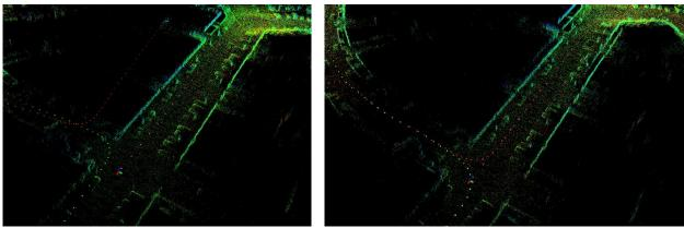
(a) Loopback detection test failed (b) Loopback detection test successful **Fig. 6 – KITTI dataset loopback detection test**
