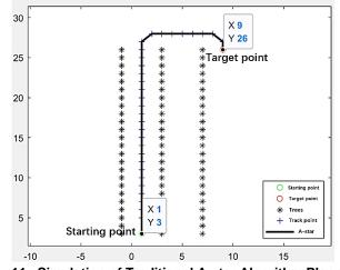
Fig. 11– Simulation of Traditional A-star Algorithm Planning
