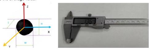
Fig. 1 - Triaxial dimensional measurement of Pak Choi seed
