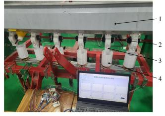
**Fig. 11 - Indoor experiment** 1 – seed box; 2 – propshaft; 3 – seed dispenser; 4 – weighting unit
