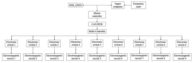
Fig. 1 – PTO protocol variable spray system components
