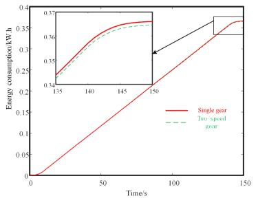
Fig. 9 - Comparison in one ploughing test cycle
