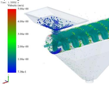
Fig. 9 - Article velocity vector diagram of simulation process
