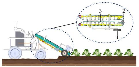
1 - profiling area; 2 - root cutting- lifting area; 3 - clamping and conveying area
