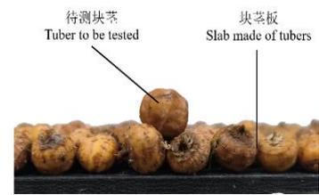
**Collision restitution coefficient test**
