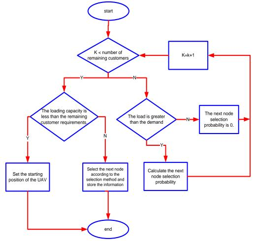
Fig. 1 – The basic process of ant colony algorithm
