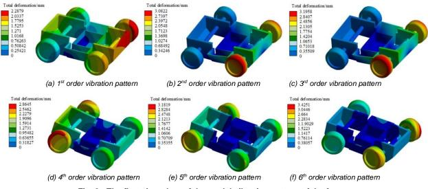
Fig. 8 - The first six orders of the modal vibration pattern of the frame
