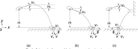
Fig. 2 - Schematic diagram of fruit movement after detachment
