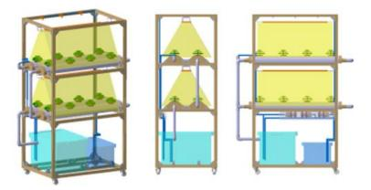
Fig. 1 - Overview of two-layer recirculating hydroponics system
