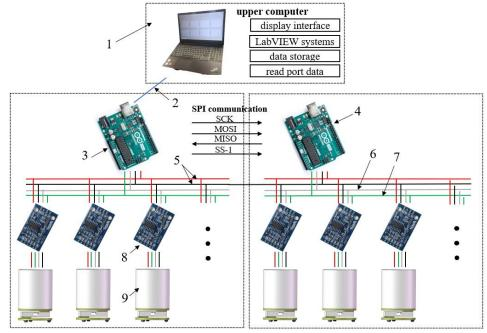
**Fig. 1 - The overall schematic diagram of the device** 1 – LabVIEW upper computer; 2 – Type-B to Type-A; 3 – Arduino master; 4 – Arduino slave; 5 – 5v power supply; 6 – SCK cord; 7 – DT cord; 8 – HX711 converter chip; 9 – weighing unit
