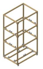
Fig. 2 – Pipelines supporting aluminum frame
