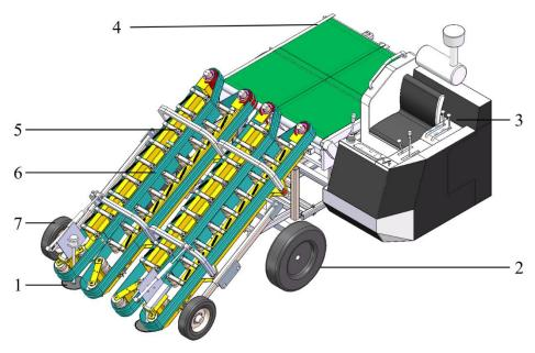
1 - root cutting device; 2 - guide wheel; 3 - cockpit; 4 - transverse conveying platform; 5 - tension pulley; 6 - clamping conveyor belt; 7 - profiling device
