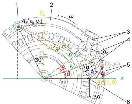
**Fig. 6 - Schematic analysis of the key parameters of the seed scraper** *1. positioning hole; 2. arc-shaped frame; 3. scraper blade* III; *4. scraper blade* II; *5. scraper blade* I; *6. hole* I.
