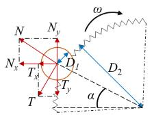
Fig. 11 - Force analysis diagram of root cutting process
