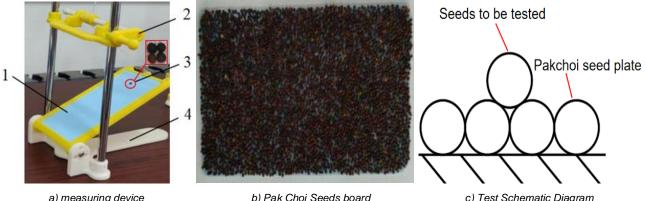
device b) Pak Choi Seeds board c) Test Schematic Diagram Fig. 4 - Test for determination of static friction coefficient between seeds
