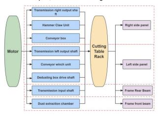
Fig. 5 - Pick up header OPTA vibration transmission path diagram
