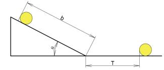
Fig. 5 - Schematic diagram of inclined plane rolling friction test measurement
