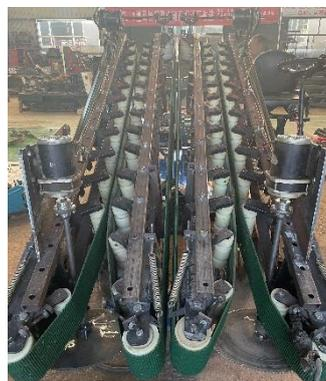
(b). Clamping conveying mechanism physical diagram
