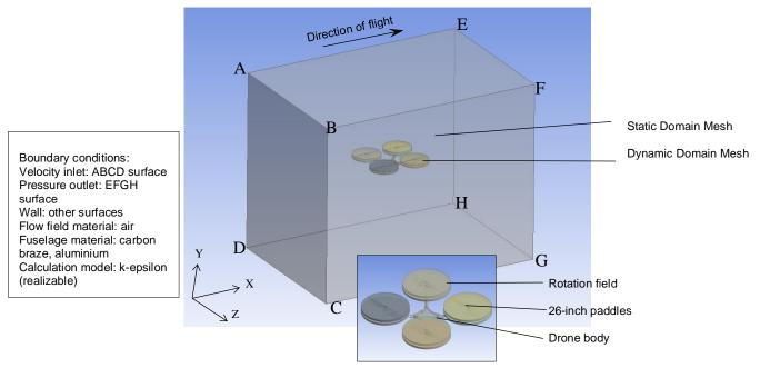
Fig. 9 - Simulation environment construction
