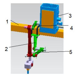
Fig. 1 - Schematic diagram of deep application mechanism 1.Main beam, 2. Front swing arm spindle seat, 3. Spray automatic control valve, 4. Left crank arm, 5. Fertilization spray needle assembly
