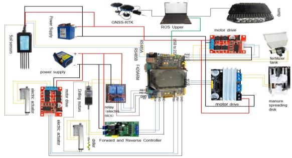
Fig. 10 - System hardware wiring diagram
