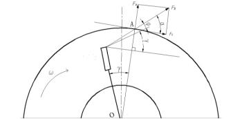
Fig. 3 - Schematic diagram of material particles impacting screen plate
