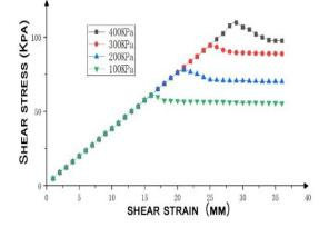
Fig. 4 – Shear Displacement-Shear Stress Relationship Curve
