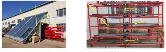
(a) (b) **Fig. 2 - (a) Solar-heat pump combined drying system;** (b) **Dynamic drying device** 1.Solar collector; 2. Dehumidification system; 3. Drying room; 4. Mesh belt drying bed; 5. Control system; 6. Drying frame; 7. Drive chain; 8. Swivel frame; 9. Drying bed; 10. Electric motor
