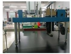
**Fig. 3 – ZJ type strain control type straight shear instrument** 1. axle; 2. base; 3. permeable stone; 4. piston; 5. gauge; 6. upper box; 7. soil sample; 8. lower box; 9. gauge; 10. gauge ring
