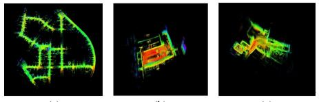
(a) (b) (c) Fig. 7 – Maps constructed by the LeGo-LOAM algorithm
