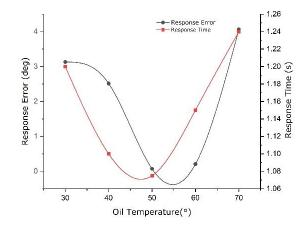
Note: Oil supply pressure 12 MPa, driving speed 8 km/h Fig. 8 - The effect of oil temperature on steering performance
