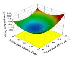
f) Intake pipe diameter and temperature difference on mixing temperature
