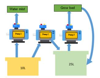
Fig. 12 – Diagram of working principle for feeding water and misting
