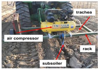
Fig.1 - Pneumatic subsoiling equipment
