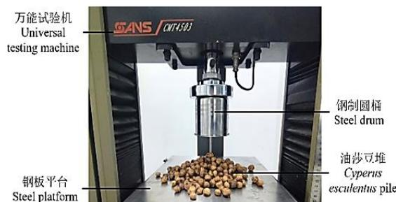
Fig. 4 – Physical Repose angle test of Tiger nut tubers
