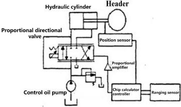
Fig. 5 - Schematic Diagram of the Header Height Measurement and Control System Based on Ultrasonic Sensors (*Yang et al., 2008*)
