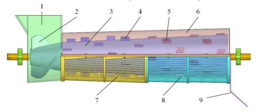
**Fig. 1 - Structural diagram of variable pitch corn threshing device** 1.feed hopper; 2.spiral blade; 3.threshing drum; 4.plate teeth; 5.D-type ribs; 6.cover plate; 7.threshing concave plate; 8.separation concave plate; 9. discharge deflector plate
