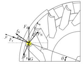
Fig. 3 - Force analysis diagram of the seed-cleaning process
