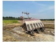
(a) Test site (b) Path-tracking test of the transplanter headland turning **Fig. 5 - Experimental scenario of curved path-tracking for the rice transplanter on the field**
