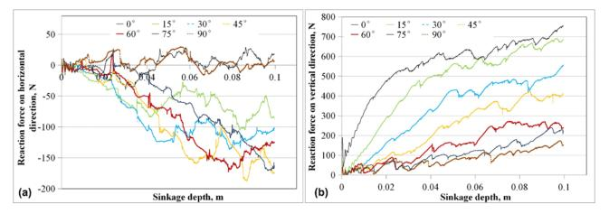
Fig. 8 – Relationship between the forces exerted on the plates and the penetration depth: (a) - in the horizontal direction, (b) - in the vertical direction
