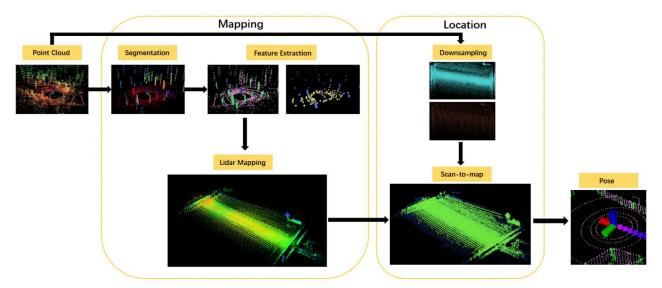
Fig. 6 - Multi-line LiDAR-based SLAM system structure diagram
