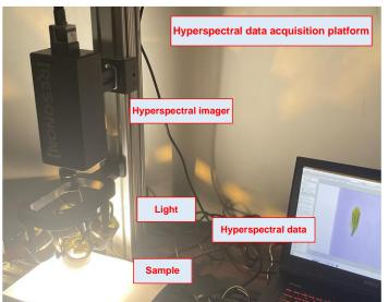
Fig. 1 - Hyperspectral data acquisition platform
