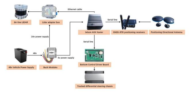
Fig. 5 – Hardware Connection Diagram of Orchard Work Robot
