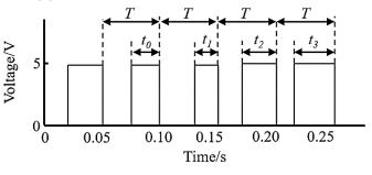
Fig. 9 – PWM digital signal
