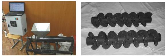
a) b) Fig. 2 - General view of the stand for the investigation of the screw conveyor (a) and a screw working body, consisting of individual blades (b)
