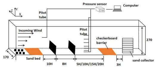
Fig. 4 - Wind tunnel test layout (unit: mm)
