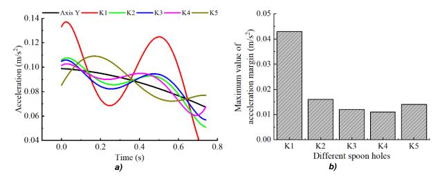
Fig. 12 - Comparative diagram of seed acceleration in the y-direction at a working speed of 2 km/h a) Acceleration change curve; b) Maximum difference of acceleration
