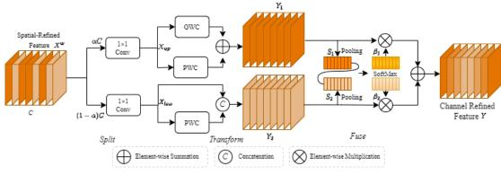
Fig. 5 - The architecture of Channel Reconstruction Unit
