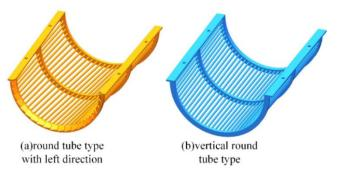
Fig. 3 - Structure of the concave plate for two mounting orientations
