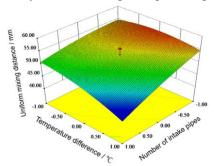
a) Effects of the axial angle of the incision and the diameter of the inlet pipe on the uniform mixing distance
