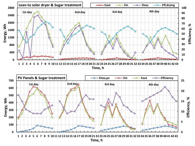
Fig. 13 – The calculated energy input (E<sub>in</sub>), energy output (E<sub>out</sub>), energy loss (E<sub>loss</sub>), and efficiency for collector, dryer, and PV for sugar treatment of slices and halves tomatoes
