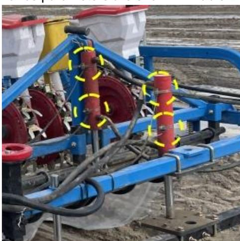
Fig. 4 - Installation diagram of Hydraulic limit sensor
