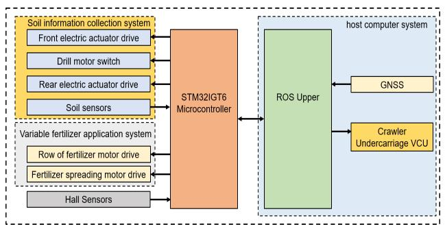
Fig. 2 - Schematic diagram of control system of variable fertilization device based on soil nutrient detection
