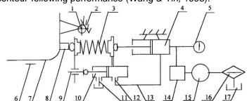
Fig. 3 - Schematic Diagram of the Hydraulic Profiling Mechanism for a Suspended Header (*Wang & Yin, 1998*) 1. Hinge; 2. Frame; 3. Buffer Spring; 4. Cylinder; 5. Pressure Gauge; 6. Profiling Plate; 7. Header; 8. Press Block; 9. Adjusting Bolt; 10. Quick Release Valve; 11. Oil Outlet; 12. Oil Inlet; 13. Pipeline; 14. Pressure Reducing Valve; 15. Oil Pump; 16. Oil Filter; 17. Oil Reservoir
