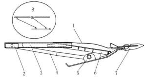
Fig. 2 - Schematic Diagram of the Floating Cutter Structure (*Li et al., 2024*) 1.Elastic Header Base Plate; 2. Mounting Plate; 3. Base Trough Plate; 4. Rotary Arm Assembly; 5. Lower Base Plate Assembly; 6. Limiting Plate Assembly; 7. Cutter; 8. Principle of Four-Bar Linkage Mechanism
