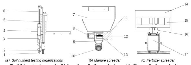
**Fig. 3 Schematic diagram of soil information collection mechanism and fertilizer application mechanism** 1. Drill; 2. Soil acquisition sensor; 3. Coupling; 4. Planetary gear reduction motor; 5. Rear electric push rod; 6. Front electric push rod; 7. Fat box; 8. Outer wheel; 9. Manure box; 10. Fertilizer can; 11. Fertilizer discharge motor; 12. Fertilizer fan leaf; 13. Fertilizer brush; 14. protected zone; 15. Manure spreader; 16. Ring flange; 17. Fertilizer motor
