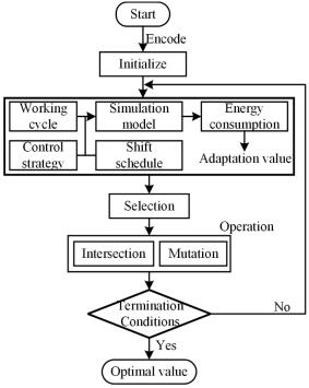
Fig. 6 - Work flow optimization of the gear ratio
