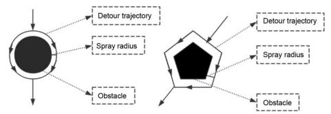
Fig. 4 - Schematic diagram of obstacle avoidance and detour for plant protection UAV
