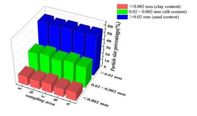
Fig. 5 – Saline soil particle size distribution
