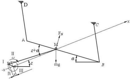
Fig. 3 - Sketch of vibrating screen motion
