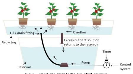
Fig. 3 – Flood and drain technique plant growing (https://www.trees.com/gardening-and-landscaping/ebb-and-flow-hydroponics)
