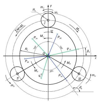
Fig. 2 - Scheme of resistance force factors affecting the rotary tiller with planetary mechanism
