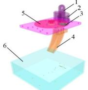
Fig. 13 - Sowing device simulation experiment 1. Brush; 2. Seed box; 3. Pak Choi seeds; 4. Seed tubes; 5. Seed tray; 6. Seed collection bin.
