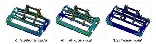
Fig. 7 - The front sixth-order modal shapes of the pickup header frame
