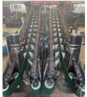
(a). Clamping conveying mechanism (b). Clamping conveying mechanism physical diagram Fig.17 - Clamping device
