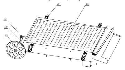
Fig. 2 - Screening device 301 - Pulley I; 302 - Crank; 303 - Connecting rod; 304 - Suspension rod; 305 - Vibrating screen
