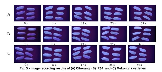
The image obtained in the image recording is then analyzed with the ImageJ application. After receiving the RGB value, the value of six rice grains is averaged to become the value of 1 sample. The calculation results of each sample are then made into a graph using Microsoft Excel software.
