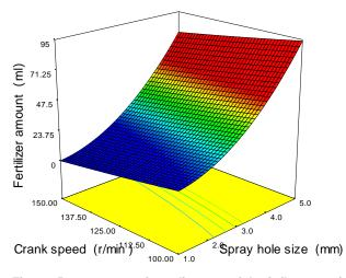
Fig. 8 - Response surface diagram of the influence of crank speed and spray diameter on fertilizer application rate
