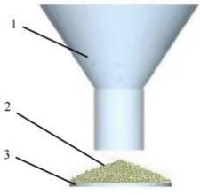
Fig. 11 - Angle of repose simulation test 1. Funnel; 2. Pak Choi seeds; 3. Chassis.
