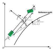
Fig. 2 - Tracking error model
