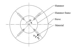
Fig. 2 - Schematic diagram of movement of material particles
