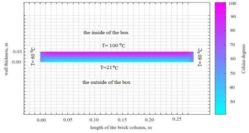
Fig. 5 - Temperature variation inside the wall (assembly) of seven bricks used to determine the coefficient of thermal conductivity (fig. 1c)
