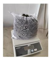
Fig. 8 – Preparation of plant material: packing in special cloth bag and weighing
