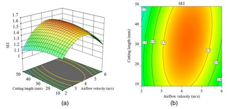
Fig. 6 - Response surface of the airflow velocity and cutting length to the separation evaluation index
