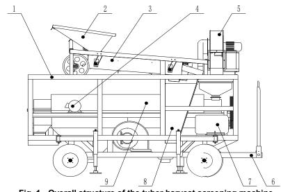
Fig. 1 - Overall structure of the tuber harvest screening machine 1 - Frame; 2 - Feeding hopper; 3 - Screening device; 4 - Screening device dynamo; 5 - Air separation unit; 6 - Hitch frame; 7 - Polishing device dynamo; 8 - Impurity removal slide; 9 - Polishing device
