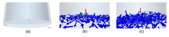
Fig. 13 – Process of impact force transmission (a) With no seed accumulation; (b) With 500 seeds accumulated; (c) With 1000 seeds accumulated
