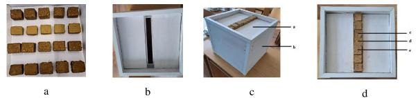
Fig. 1 - The components of the experimental system a - bricks made of composite material; b - box with a slot made for moving the bricks; c - bricks mounted in the slot of the box with the heat source, ready for measurement; d - measurement points on the brick wall.
