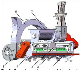
**Fig. 2 - Straw forage harvester pick up header** 1. Hammer Claw Device; 2. Conveying device; 3. Transmission; 4. Right side panel of the frame; 5.Conveyor box; 6. Ejection device; 7. Dust box.
