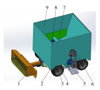
Fig. 1 - Structure of the supplemental feed pusher 1. Cleaning device; 2. Frame; 3. Wheel encoder; 4. Rolling wheel; 5. Feeding plate; 6. Motor; 7. Leak-proof baffle; 8. Feeding screw; 9. Silo
