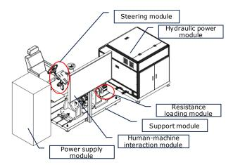
Fig. 1 - Structure drawing of tractor E-HCSS
