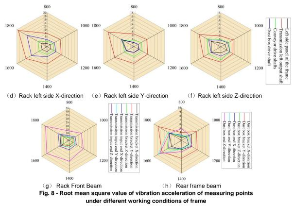
$(a \sim c)$  Root-mean-square value of vibration acceleration at the right side of the frame.  $(d \sim f)$  Root-mean-square of vibration acceleration at the left measurement point of the rack. (g) Root-mean-square value of vibration acceleration at measurement points on the front beam of the frame. (f) Root-mean-square value of vibration acceleration at the rear beam measurement point of the frame.
