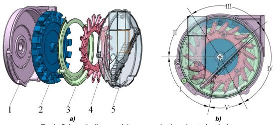
Fig. 1 - Schematic diagram of the spoon-wheel seed-metering device
