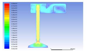
Fig. 7 - Velocity cloud of the optimized vacuum unit
