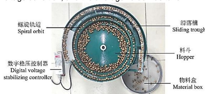
Fig. 10 – Electromagnetic vibration hopper test
