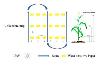
Fig. 9 - Schematic layout of water-sensitive test strips
