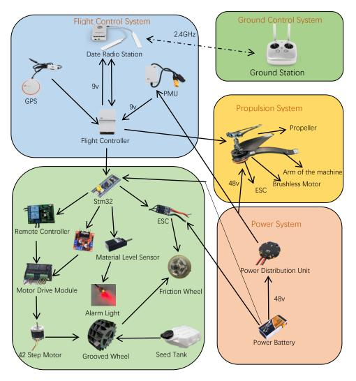
Fig. 4 - Components of the UAV and the workflow of each system
