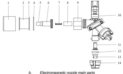
Electromagnetic nozzle main parts
