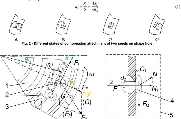
Fig. 3 - Schematic diagram of the forces on the excess seeds before enters the clearing area 1. seeding plate; 2. excess seeds; 3. groove; 4. shape hole; 5. forces of excess seed z-axis direction.
