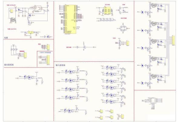
Fig. 9 - Schematic diagram of the driver circuit board
