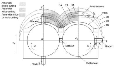
Fig. 2 - Cutting area diagram of disc cutter
