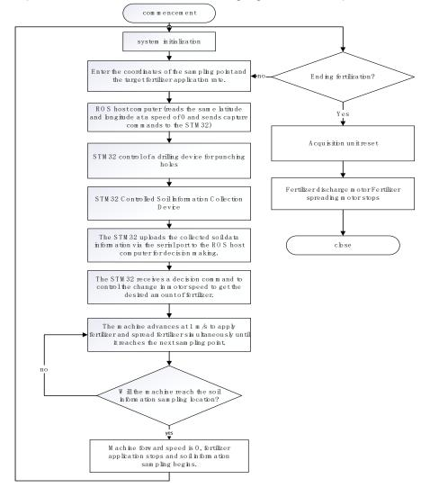
Fig. 11 - Flow chart of variable fertilization control based on soil nutrient content detection
