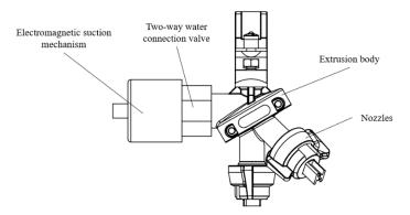
Electromagnetic nozzle assembly diagram а.
