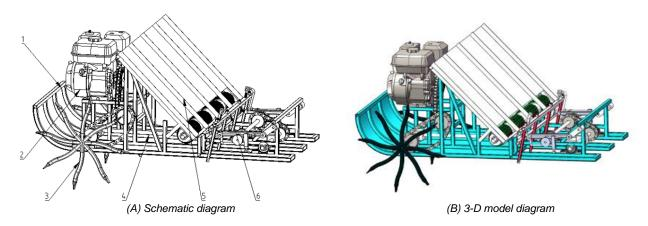
**Fig. 1 – The overall structure of 2ZQS-4 rice transplanter** 1-frame; 2-engine; 3-paddy wheel; 4-transmission system; 5-rice paddy; 6-rice transplanter mechanism.
