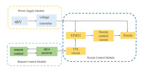
Fig. 3 - Control system composition
