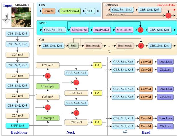
Fig. 2 - CA-YOLOv8 network structure
