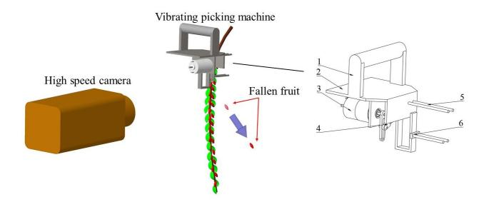
Fig. 1 - Schematic diagram of fruit drop (1) hand shank, (2) shell, (3) DC motor, (4) a crank-swinging lever, (5) clamping rob, (6) vibrating rod.
