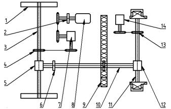
Fig. 2 – 2ZQS-4 rice transplanter transmission system schematic diagram 1-Paddy wheel; 2-Electromagnetic clutch; 3-Wheel shaft; 4-Sprocket; 5-Reversing reducer; 6-Electromagnetic clutch; 7-Reversing reducer; 8-Engine; 9-Seedling box; 10-Main drive shaft; 11-Transplanting mechanism drive shaft; 12-Reversing reducer; 13-Sprocket; 14-Transplanting mechanism.
