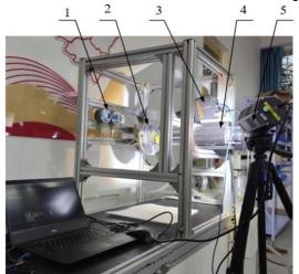
Fig. 4 – Test bench and test seeds 1. Digital display precision pressure gauge; 2. Pneumatic precision seed discharger; 3. High speed camera; 4. Servo motor; 5. LED flash light
