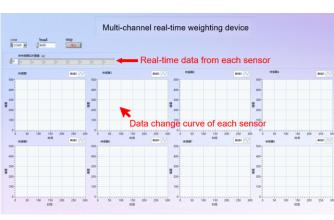
Fig. 4 - The LabVIEW front panel interface
