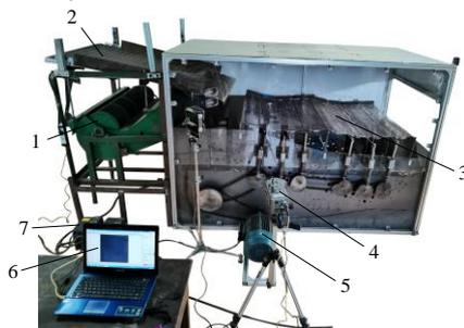
Fig. 6 - Cleaning device of bionic screen
