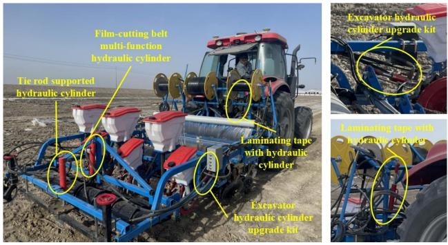
Fig. 7 - Installation diagram of hydraulic cylinder
