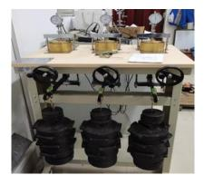
Fig. 4 - WG type single lever consolidation instrument
