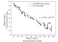
Fig. 6 – Boundary fitting of one-side stacking angle
