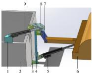
**Fig. 7 - Sketch of the structure of the cleaning device** 1. Mounting bracket; 2. Frame; 3. Fixed plate; 4. Centre shaft; 5. Electric actuator 1; 6. Brush roller; 7. Connecting plate; 8. Rotating bracket; 9. Electric actuator 2
