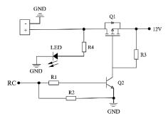
Fig. 6 – Electronic switch circuit diagram
