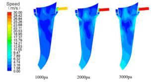
Fig. 6 - Front velocity nephogram under different wind pressures
