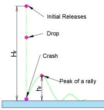
Fig. 7 - Schematic diagram of the collision recovery coefficient determination test
