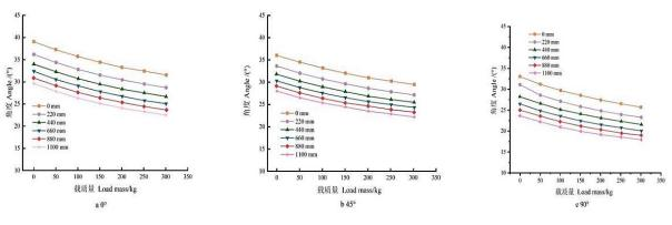
Fig. 11 - Simulation results of orchard platform tipping (a) 0°; (b) 45°; (c) 90°
