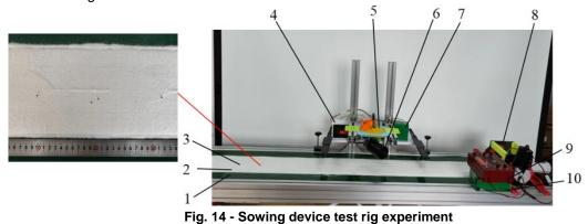
Conveyor belt; 2. Sand; 3. Pak Choi seeds; 4. Seeding Controller; 5. Seed-metering device; 6. Electrical machinery;
