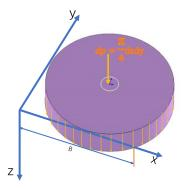
Fig. 2 - Stress under uniform circular load corner
