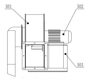
**Fig. 4 - Air separation unit** 501 - Fan casting; 502 - Air separation unit dynamo; 503 - Support
