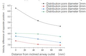
Fig. 15 - Influence of different distribution pore diameter on velocity difference in the opposite position
