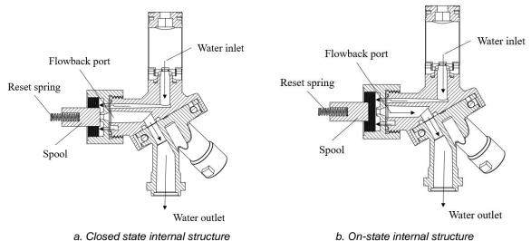
Fig. 3 – Internal structure of two-way water connection valve and spray body section
