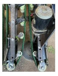
(a). 1 - root cutting device motor; 2 - saw-tooth disc cutter; 3 - clamping device. (b). The physical diagram of the root cutting device **Fig. 9 - Root cutting device**
