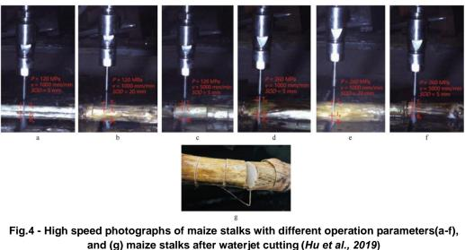
T represents the top point of the maize stalks; B represents the bottom point of the maize stalks; J represents the deepest point of waterjet.
