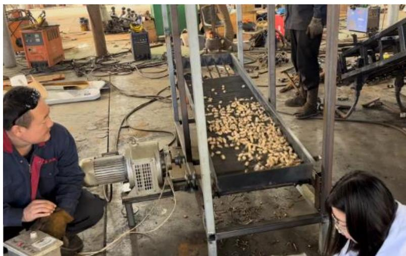
Fig. 8 – Cleaning screen device test bench
