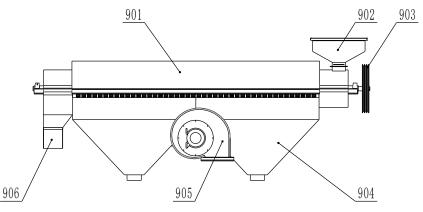
Fig. 5 - Polishing device
