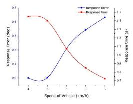
Note: Oil temperature 50°C, oil supply pressure 12 MPa Fig. 10 - The effect of speed on steering performance
