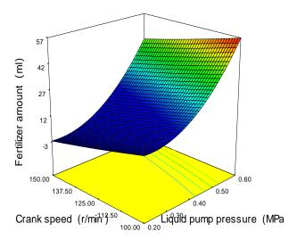
Fig. 7 - Response surface diagram of the influence of crank speed and liquid pump pressure on fertilizer application rate
