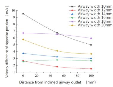
Fig. 12 - Influence of different airway widths on velocity difference in the opposite position
