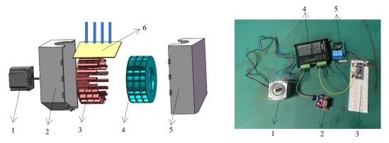
Fig. 7 - Seed Discharger Structure Diagram
