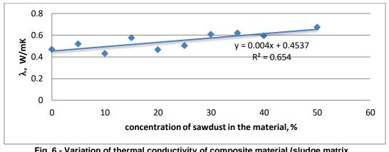
Fig. 6 - Variation of thermal conductivity of composite material (sludge matrix with sawdust insert) with the concentration of sawdust insert
