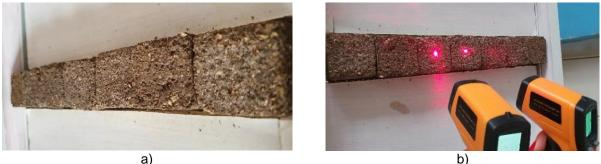
Fig. 2 - Measuring the external temperature on bricks a - laying of bricks b - temperature measuring devices.
