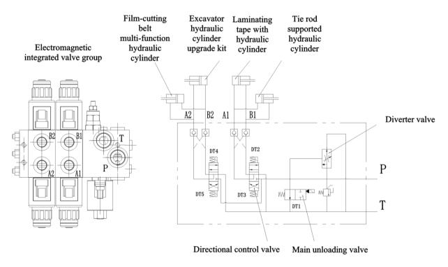
Fig. 11 - Hydraulic control schematic
