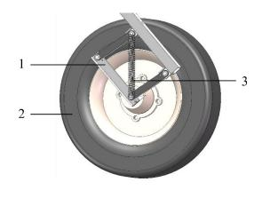
Fig. 5 - Schematic diagram of the structure of the profiling device 1 - profiling brackets; 2 - profiling wheel; 3 - profiling sprung
