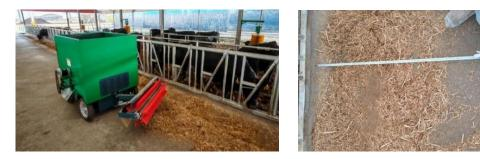
Fig. 9 - Supplemental feeding pusher discharging test (a) Test Scene (b) Measurement process
