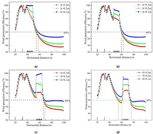
Fig. 10 – Chart of wind protection efficiency and effective protection distance: a) D=5H; b) D=10H; c) D=15H; d) D=20H.
