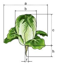
a - expansion degree; b - diameter; c - plant height; h - rhizome length; r - rhizome diameter Fig. 1 - Determination of geometric characteristics of Chinese cabbage
