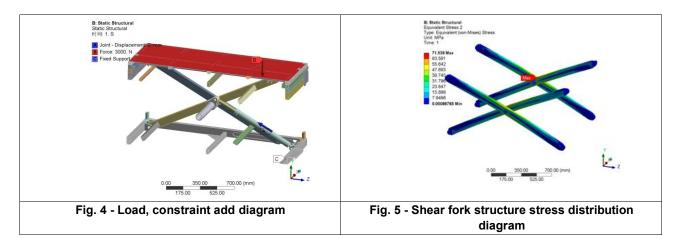
According to the stress distribution of the diagonal support and support rod of the scissor structure. The maximum stress on the system is calculated to be 71.539 MPa, as shown in Figures 5 and 6, observed in Part B. The load acting on the cylinder causes a lower stress on the lower scissor section A.
