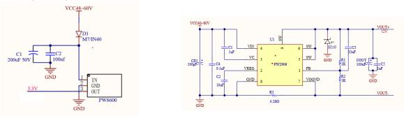
Fig. 4 - Circuit diagram of the power supply module of the control system
