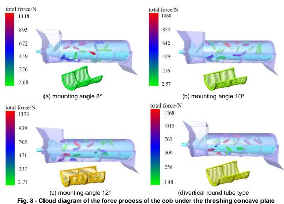
with different installation angles of the round tube
