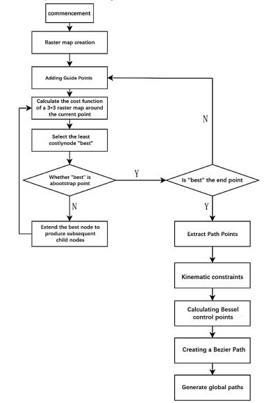
Fig. 14 – Flowchart of Improved A-star Algorithm Based on Constraint Bessel Curve
