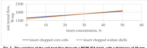
Fig. 7 - The variation of the unit heat flow through a MCMLIDA brick, with a thickness of 30 mm, in the version with an insert of chopped corn cobs and in the version with an insert made of chopped walnut shells
