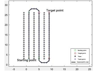
Fig. 12 – Simulation of Improved A-star Full Coverage Path Planning Algorithm
