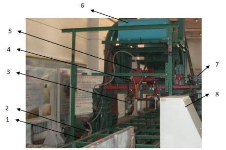
Fig. 2 - Test bench of the crank rocker deep application mechanism 1. Motor that drives the pump, 2. Piston pump, 3. Fertilizer spraying needle, 4. Crank, 5. Self-controlled spray system, 6. Fertilizer box, 7. Motor that drives the sprocket, 8. Frequency converter
