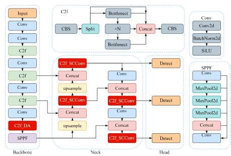
Fig. 6 - Improved YOLOv8n network structure
