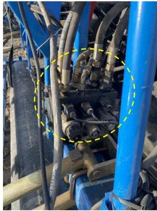
Fig. 6 - Installation diagram of Electromagnetic integrated valve group
