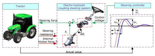
Fig. 3 - Control principle diagram of E-HCSS
