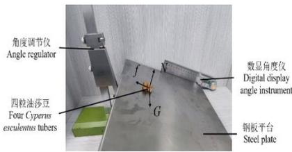
Fig. 1 – Static friction coefficient measurement
