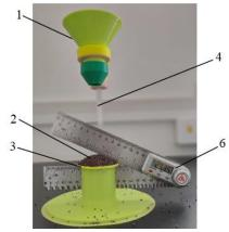
Fig. 8 - Angle of repose determination test
