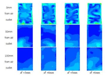
Fig. 14 - Local velocity nephogram of seed guide device
