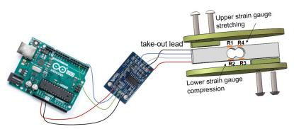
Fig. 3 - Strain gauge pressure sensor working principle diagram
