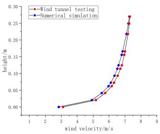
Fig. 6 – Comparison of wind speed profiles from wind tunnel experiments and numerical simulations
