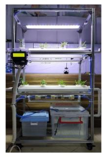
Fig. 11 – Fully assembled IoT hydroponic system
