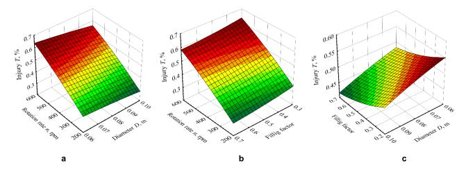
Fig. 4 - Response surface of the magnitude of damage to the pea grains depending on: a) T = f(D; n); b)  $T = f(n; \psi)$ ; c)  $T = f(\psi; n)$
