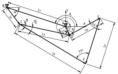
Fig. 4 – Closed-loop vector diagram of rice-planting mechanism
