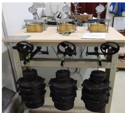
Fig. 4 - WG type single lever consolidation instrument
