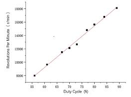
Fig. 6 - Relationship between nozzle speed and PWM duty cycle
