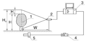
Fig. 6 – Schematic Diagram of the Header-Height Adjustment System for a Soybean Harvester (*Wu et al., 2017*) 1.Crop to be measured; 2. CCD Camera; 3. Computer; 4. Potentiometer; 5. Harvester Cutting Device
