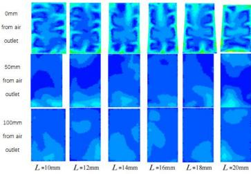
Fig. 11 - Local velocity nephogram of seed guide device
