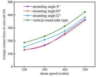
Fig. 9 - Variation of contact force of corn cob at different round tube mounting angles
