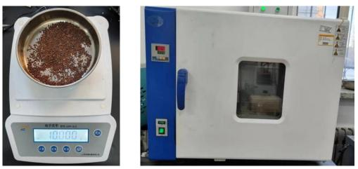
Fig. 3 - Moisture content testing device
