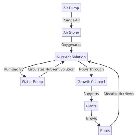
Fig. 2 – Nutrient film technique plant growing diagram
