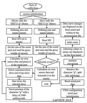
Fig. 5 - Overall workflow of the LabVIEW system
