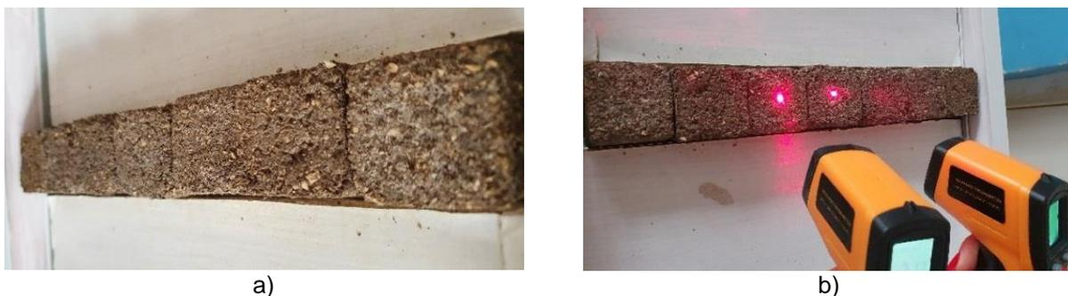
**Fig. 2 - Measuring the external temperature on bricks**
