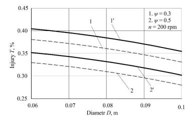
Fig. 8 - Dependences of damage to the grain material T, %, caused by the screw working element (a solid line) and a bladed one (a dashed line) on the diameter of the guide pipe D at different conveyor filling coefficients  $\psi$
