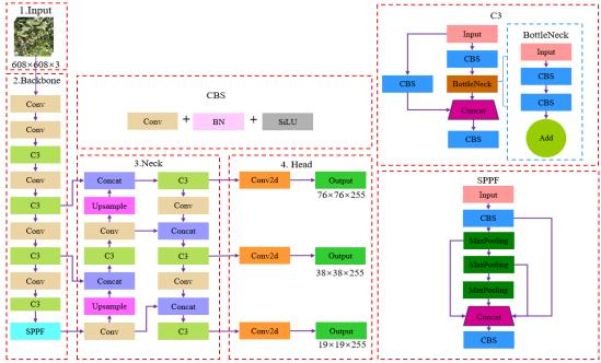
Fig. 1 - Network structure of YOLOv5s
