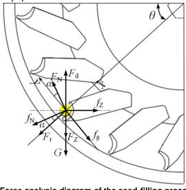
Fig. 2 - Force analysis diagram of the seed-filling process
