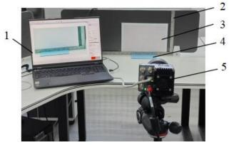
Fig. 6 - Collision restitution coefficient measurement test 1. Computer; 2. Scale; 3. Grid paper; 4. PLA material; 5. High-speed photography camera.
