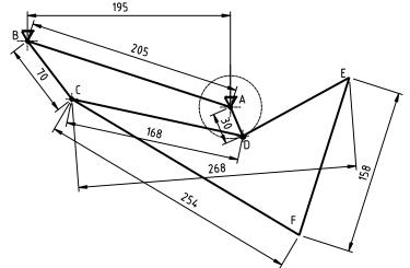
Fig. 3 – Schematic diagram of rice-planting mechanism
