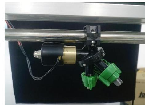
Fig. 11 – Electromagnetic nozzle physical picture
