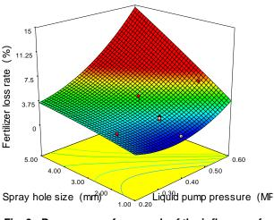
Fig. 9 - Response surface graph of the influence of spray hole diameter and liquid pump pressure on fertilizer loss rate
