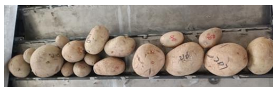
Fig. 10 - Single movable rotating plate covered with potatoes
