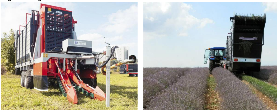
Fig. 5 - Italy RIBERI SALIUNCA lavender harvester
