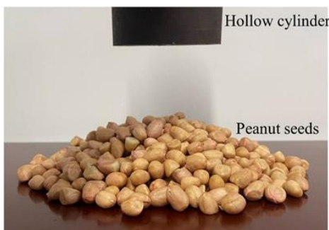
Fig. 3 - Angle of repose physical test
