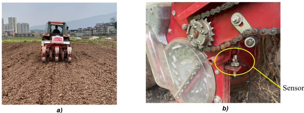
Fig. 4 - Field Experiment a) Experimental seeder; b) Sensor mounting position
