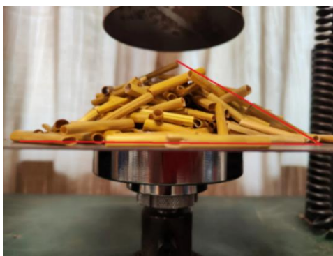
Fig. 4 - Physical test of the angle of repose by cylinder lifting method
