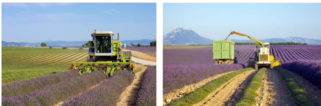
Fig. 3 - German CLAAS JAGUAR 950 forage harvester
