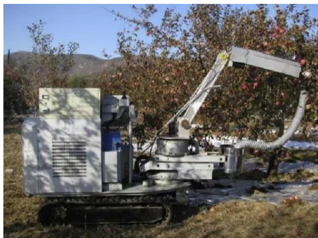
Fig. 1 - Five-degree-of-freedom apple picking robot
