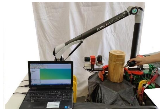
Fig. 10 – Profile measurement with RA7525SE-1005
