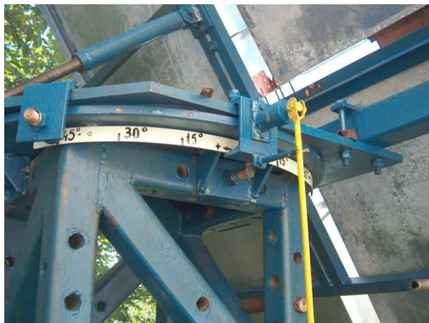
Fig. 3 – Angle indicator in horizontal plane
