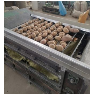
Fig. 6 - A full load of grading device
