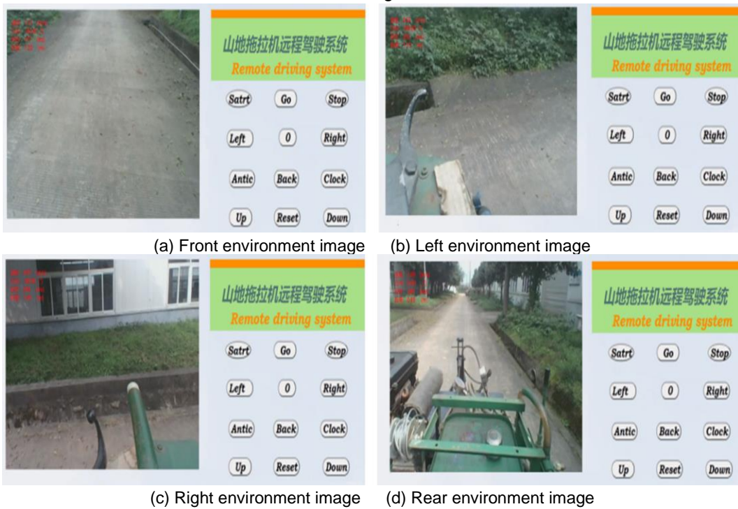
Fig. 11 - Image acquisition of the surrounding environment of the chassis
