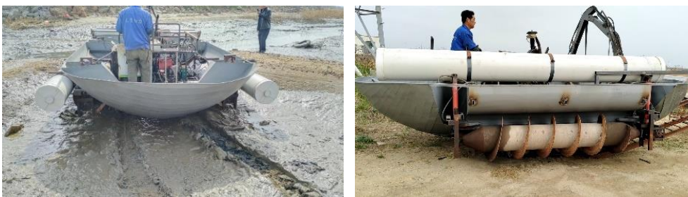
Fig.10 - Field test of twin-spiral propeller traveling device
