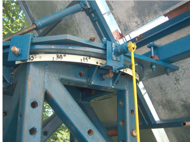
Fig. 3 – Angle indicator in horizontal plane
