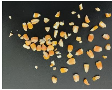
Fig. 3 - Example of corn kernel breakage
