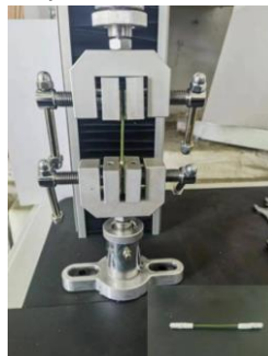
Fig. 2 - Measure the breaking force of the stem with the universal tensile testing machine
