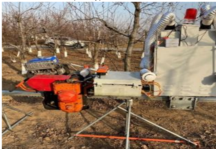
Fig. 9 - Hilly orchard frost protection smoke machine
