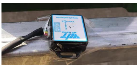
Fig. 3 - Installation position of inclination sensor
