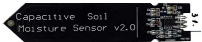
Fig. 1 - Capacitive soil moisture sensor
