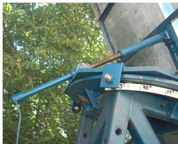
Fig. 2 – Tie rod for changing the angle of inclination of the collector in the vertical plane
