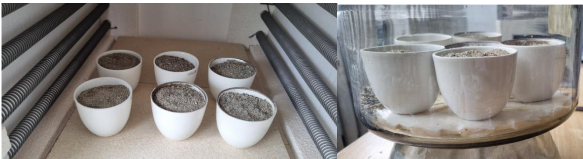
Fig. 3 – Soil samples in the oven and exicator
