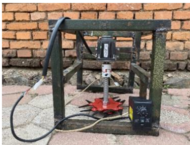
Fig. 5 - Corn straw cutting and crushing tester
