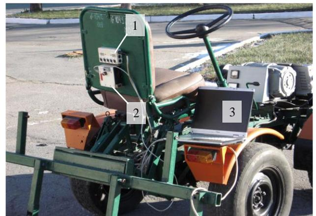
Fig. 5 - Installation of the ADC (1), the power supply (2) and the computer (3) on the tractor
