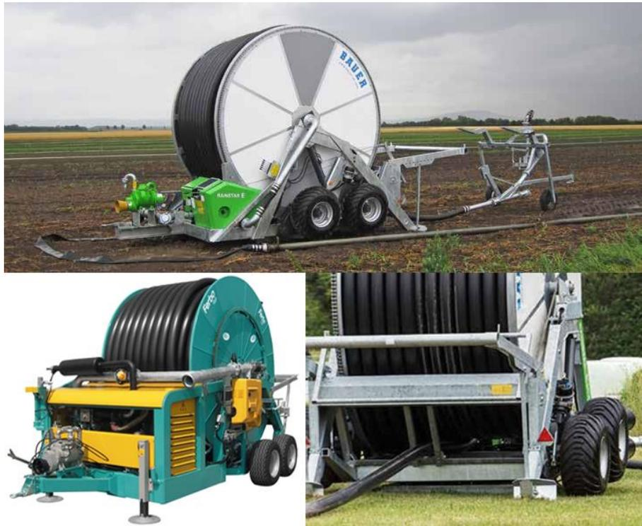
**Fig. 1 - Drum and hose irrigation system**
