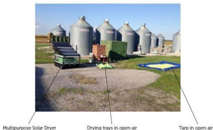
**Fig. 5 - Comparative test of multipurpose solar dryer (left), drying tray in open-air (centre), and tarp in open-air (right) (Ileleji et al., 2017)**
