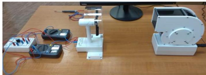
**Fig. 2 – The experimental laboratory system Windtrainer Junior**
