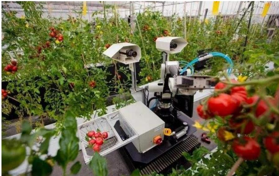
**Fig. 3 - Crawler-type greenhouse working vehicle robot**
