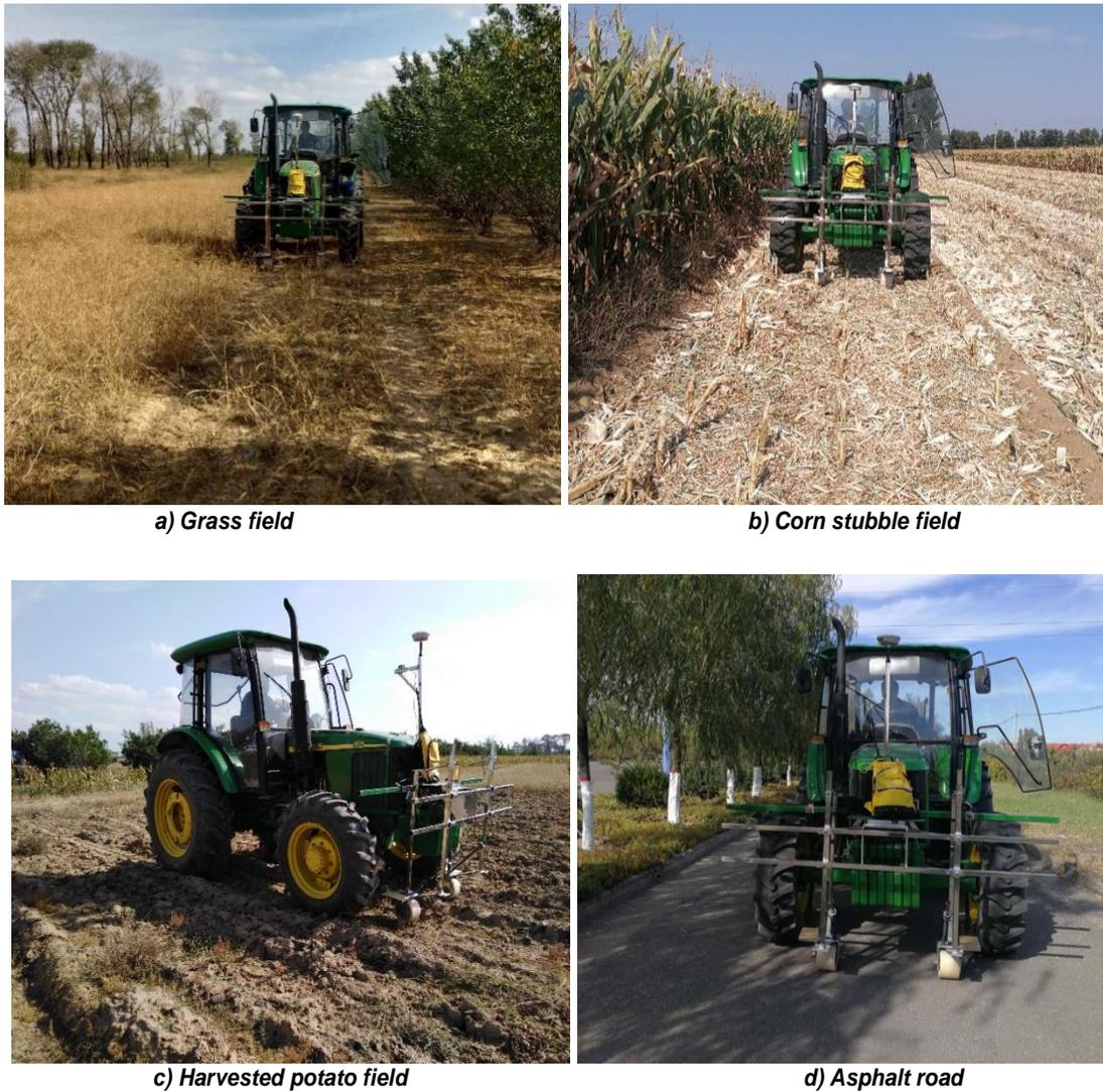
Fig. 2 - Agricultural field and asphalt road profiling measurement
