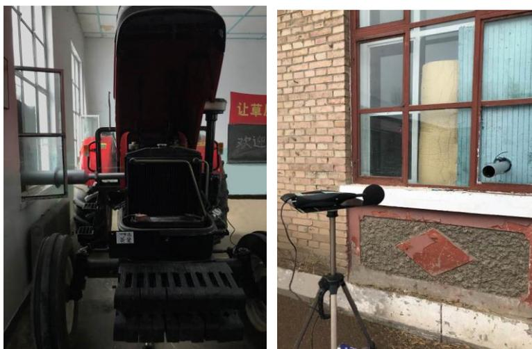
a) Exhaust noise test of coupled muffler
