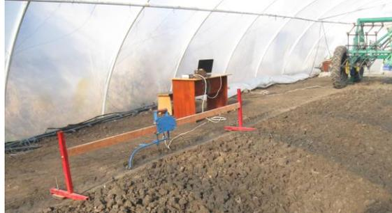
**Fig. 4 - A hardware-measuring complex for profiling the irregularities of a constant tramline traces**
