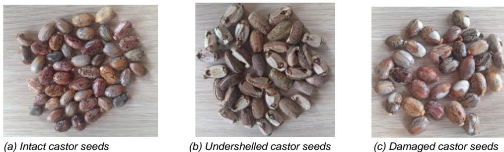
Fig. 10 - Shelling effect of the testbed
