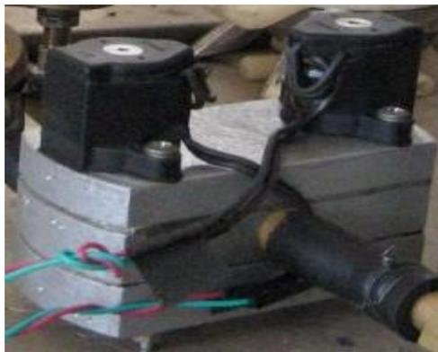
**Fig. 9 – General view of the experimental pneumo-electromagnetic pulsator of pairwise interaction**
