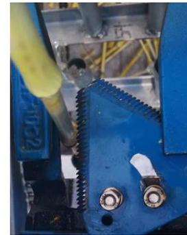
Fig. 5 - Adjustment of blade oblique angle
