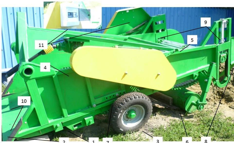
**Fig. 2 – General view of the machine for harvesting root crops and onions, equipped with a separating rod elevator with adjustable blade inclination angle and receiving plough share for digging/collecting root crops and bulbs**
