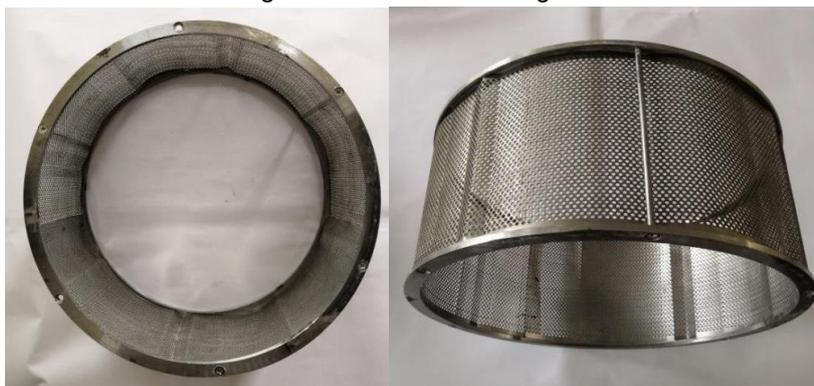
Fig. 4 – Airfoil-triangle sieve
