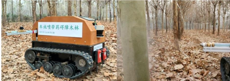
Fig. 1 - The spray system of forest barrier treatment
