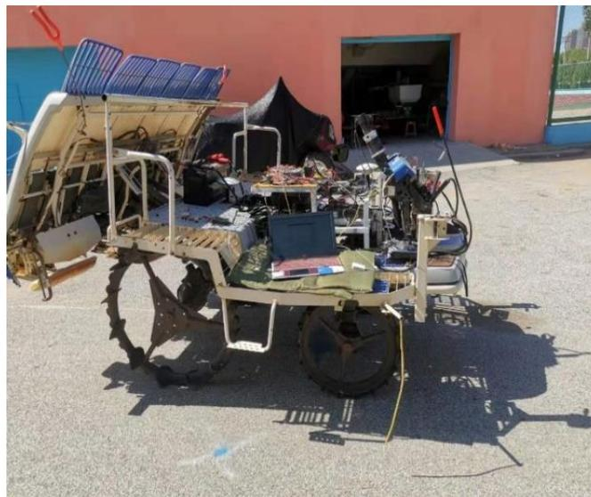
Fig. 2 - The actual vehicle test of the rice transplanter
