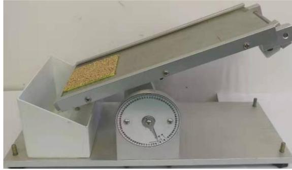
**Fig. 2 - Friction coefficient tester**
