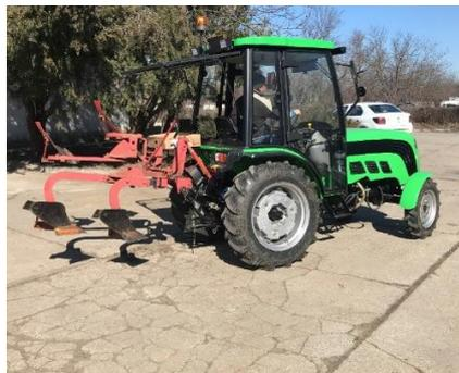
**Fig. 1 - Experimental model of electric tractor with plough mounted on**
