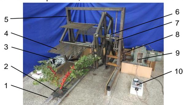
**Fig. 2 – Eccentric swing combing mechanism**
