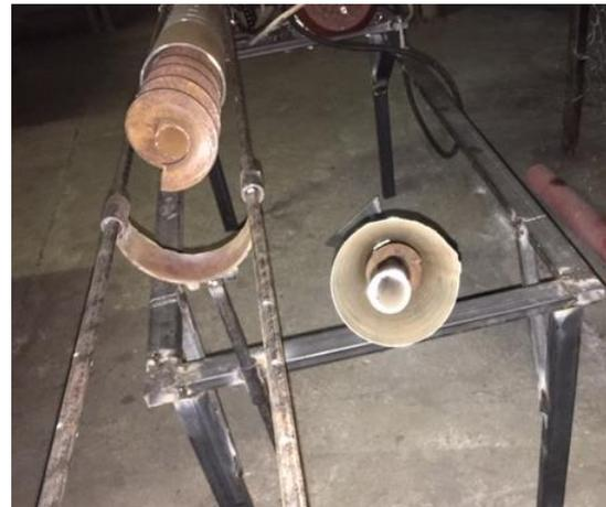
Fig. 3 - A stand for the study of telescopic screw conveyors in a disassembled state
