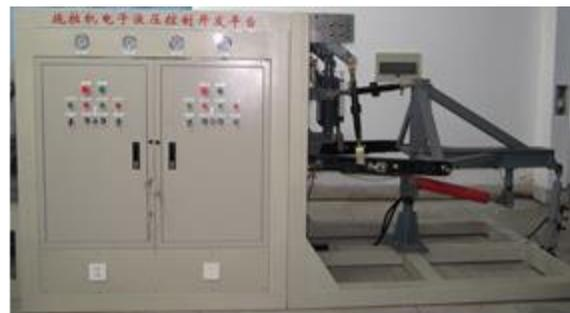
(b) Tractor electro-hydraulic control test bench
