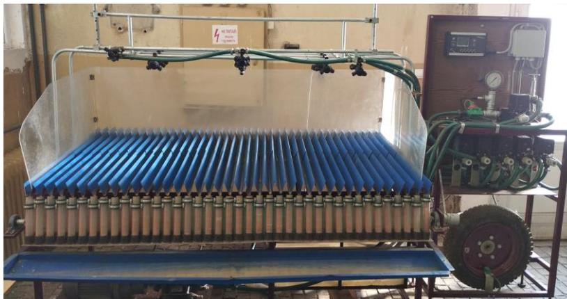
Fig. 1 - Experimental stand of spreader boom system
