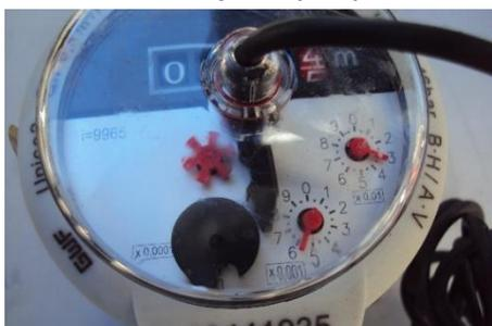
Fig. 10 - Measuring water consumption at the TLUD gasifier
