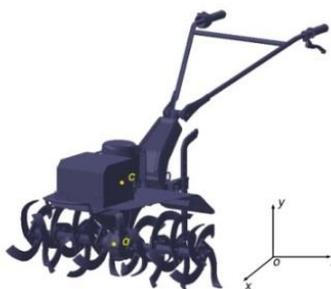
**Fig. 7 - Three-dimensional model of the electric mini-tiller**
