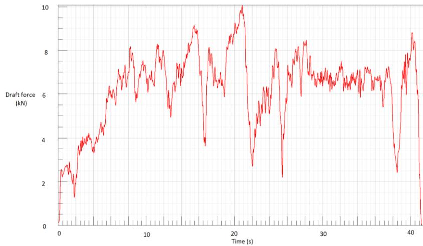
Fig. 2 - Draft force evolution for 1.1 m/s and 0.2 m depth ploughing test
