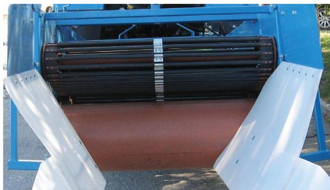
Fig. 1 – Bed-forming device of the Z-653/1 onion harvester, "Krukowiak", Poland
