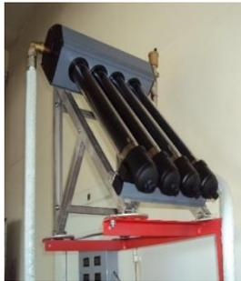
Fig.4 - Solar thermal panel with thermal sensor (S1)
