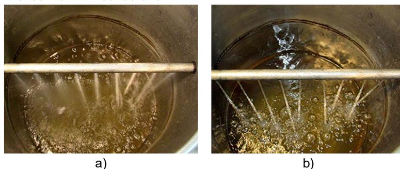
**Fig. 5 - The outflow of the air-water mixture into the bioreactor at a frequency of the pump impeller revolutions of 2720 rpm with aeration at an air pressure of 1.5 bar and (a) and without aeration (b)**
