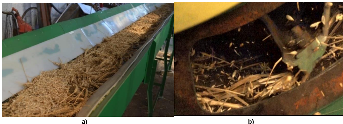
Fig. 2 – a) laboratory feed conveyor with stripped heap of winter wheat; b) high-speed shooting frame of the threshing process
