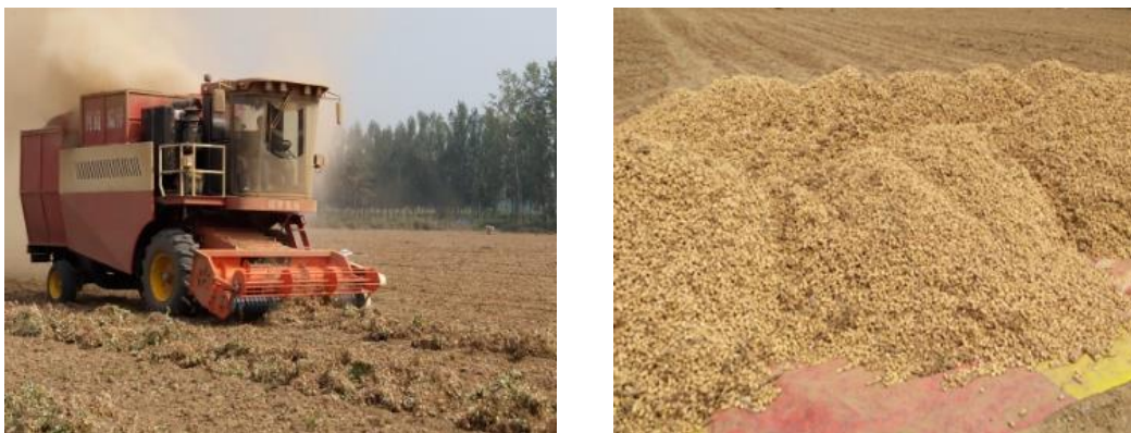
Fig. 10 - Field test process and cleaning effect of combine harvester for peanut picking-up
