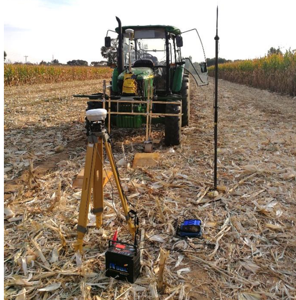
Fig. 4 - Field profiling validation test
