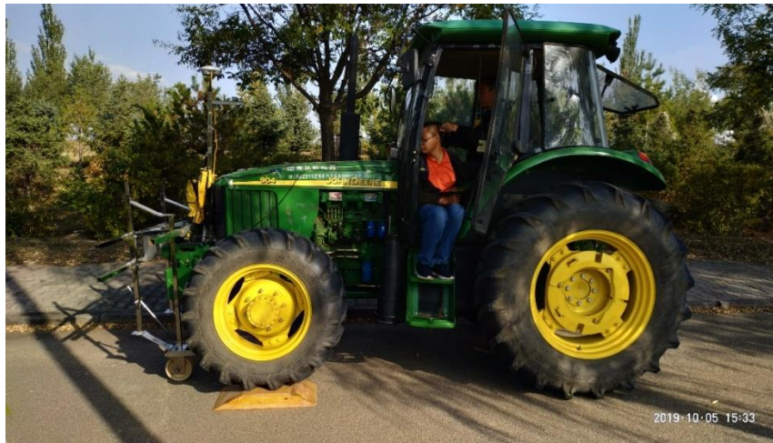
Fig. 5 - Asphalt road profiling validation test
