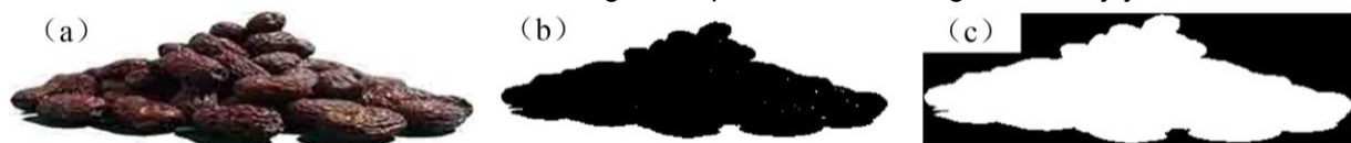
Fig. 3 - Image-processing procedure for determining the angle of repose (a) Original image; (b) Morphological processing; (c) Contour extraction and fitting
