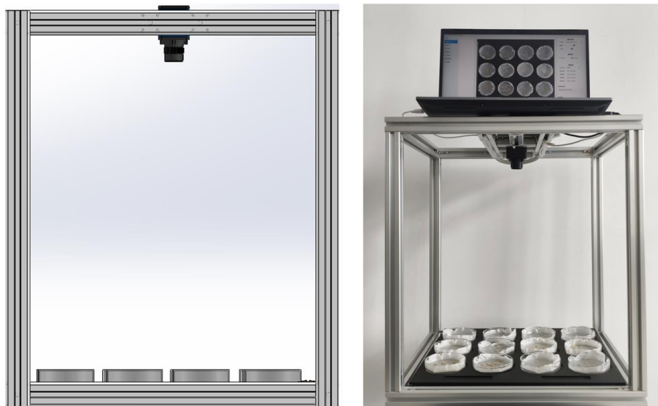
Fig. 1 - High-throughput image acquisition system for germinated seeds
