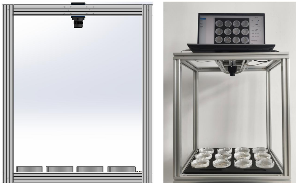
Fig. 1 - High-throughput image acquisition system for germinated seeds
