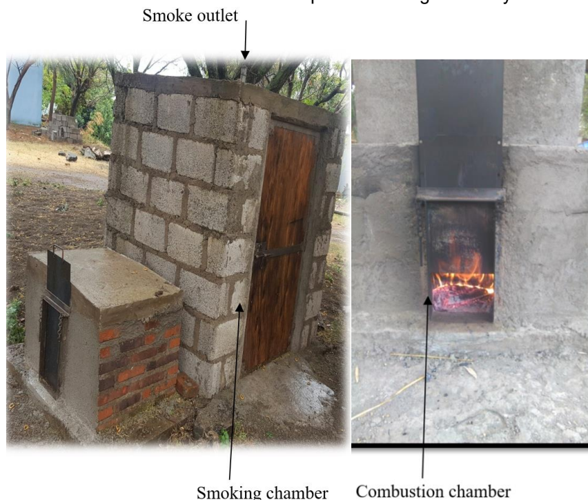
Fig. 4 - Stationary or fuelwood fish smoking technology
