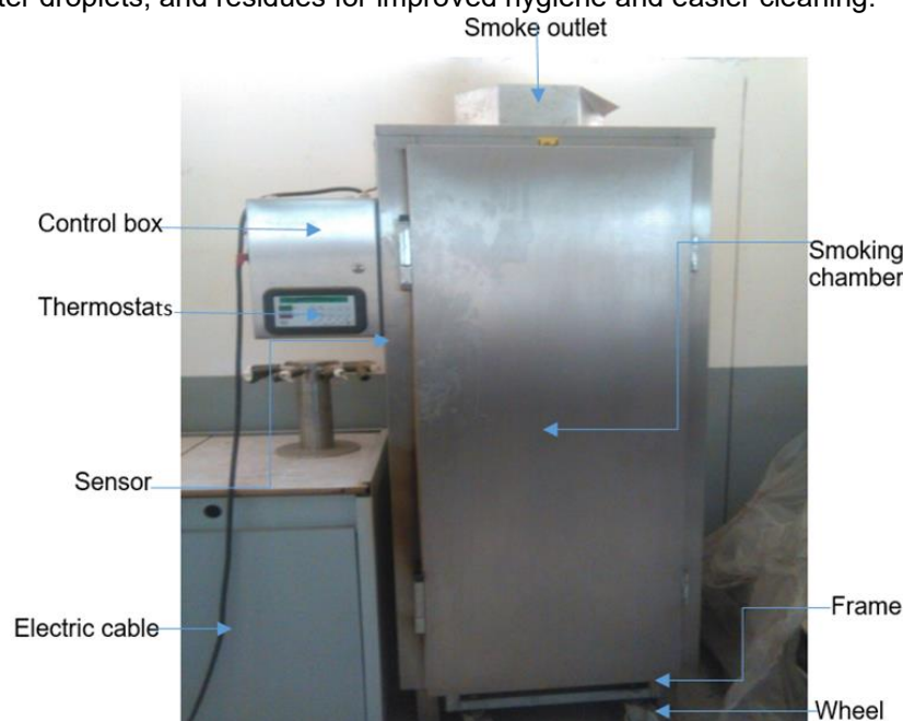
Fig. 1 - Mobile or electric fish smoking technology
