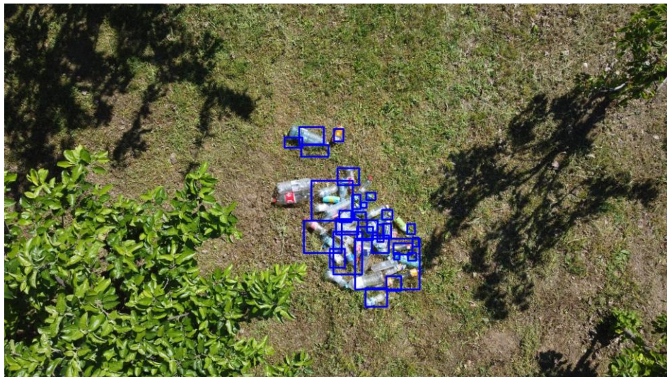
Fig. 8 - Output of the OpenCV change detection pipeline. Overlapping bounding boxes are visible due to the absence of Non-Maximum Suppression (NMS). Detection reliability under controlled conditions was approximately 72% (29 of 40 evaluated acquisitions) (original figure, produced by the authors)
