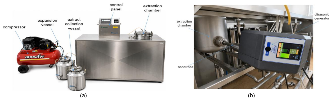
Fig. 2 - Hybrid extraction equipment: (a) front view of the TIMATIC Duo extraction system; (b) rear view showing the Hielscher UP400St ultrasonic generator
