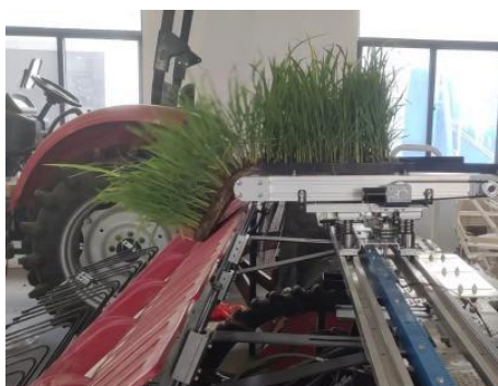
(c) Seedlings falling into seedling platform
