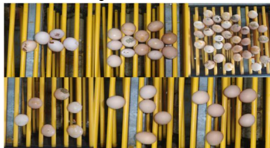
Fig. 1 - Representative images of the good, damaged, and dirty egg classes collected under conveyor-belt conditions
