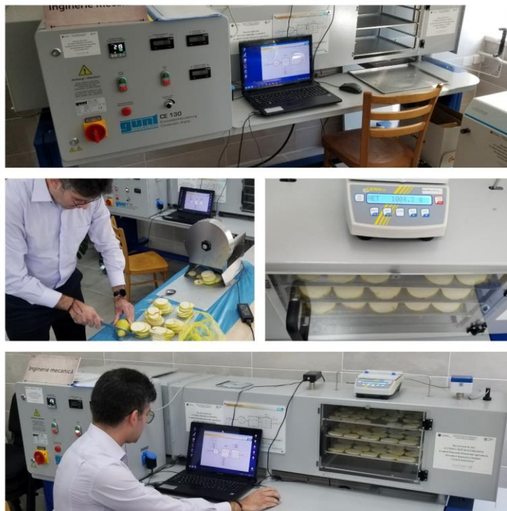
Fig. 1 - Experimental setup of the GUNT CE130 convective dryer, including sample preparation, instrumentation, and data acquisition system
