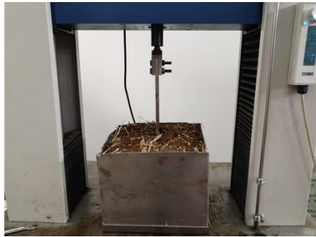
Fig. 6 - Shear test of root-soil complex
