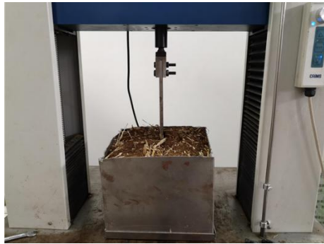
Fig. 6 - Shear test of root-soil complex
