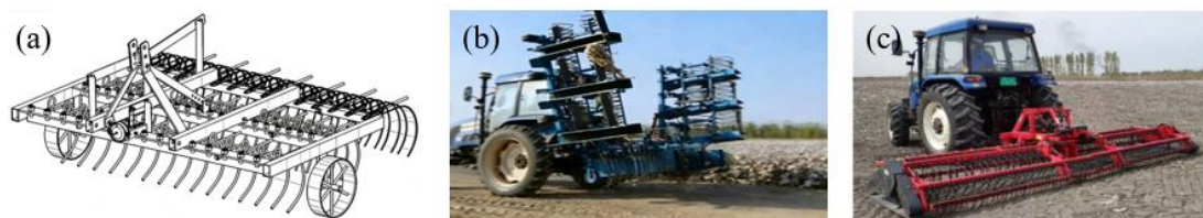
Fig. 6 – Closely Arranged Spring-Tooth Residual Film Recovery Machine
