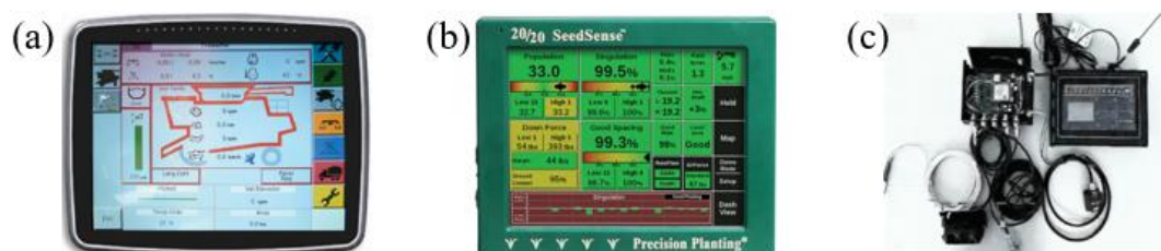
Fig. 7 – Key Component Monitoring System for Residual Film Recovery Machines
