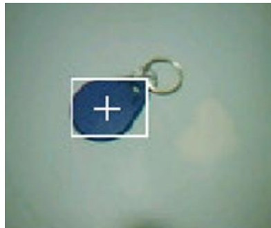
Fig. 3 - Example of color blob detection with centroid visualization
