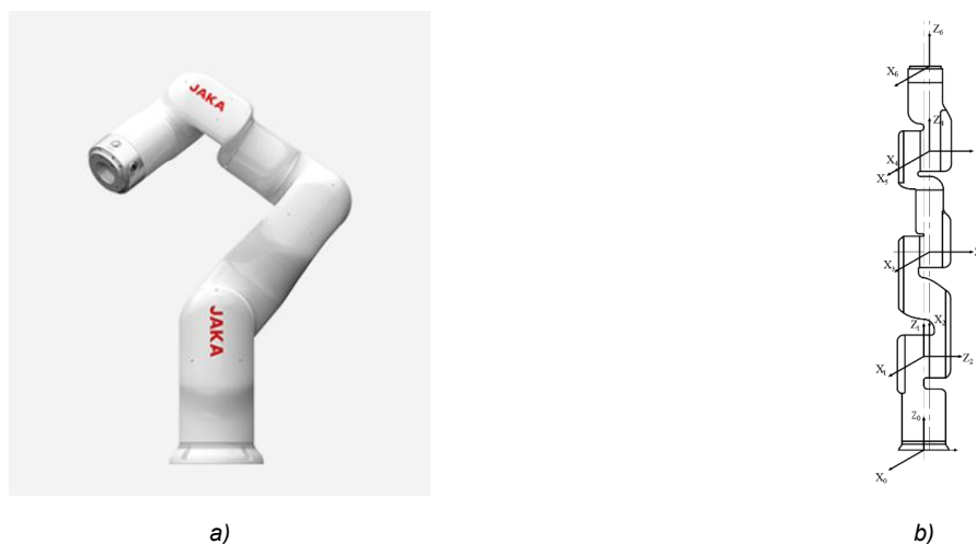
Fig. 1 – Six-axis collaborative manipulator: (a) manipulator model; (b) modified D–H coordinate system
