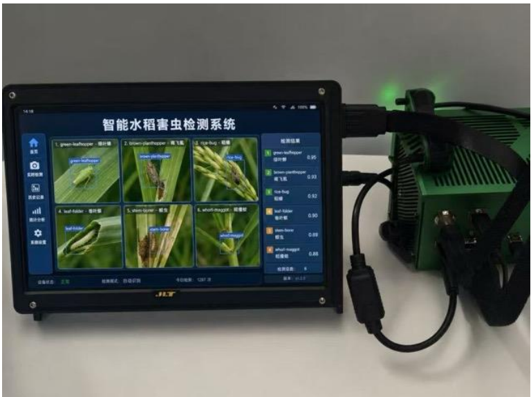
Fig. 11 - Jetson Nano deployment interface of the rice-pest detection system
