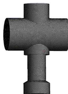
Fig. 4 - Fluid domain mesh division
