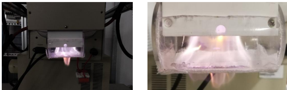
Fig. 3 - Phenomenon of gliding arc discharge seed treatment
