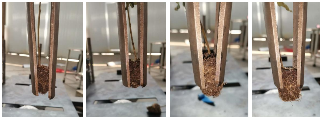
Fig. 11 - Multi-angle photographs of the flexible end-effector gripping the seedling soil plug
