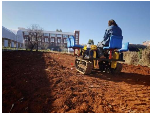
Fig. 8 - Straight-line travel deviation test of the transplanter
