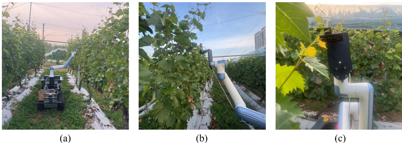
Fig. 10 - Field application of the vineyard inspection robot for grape disease detection
