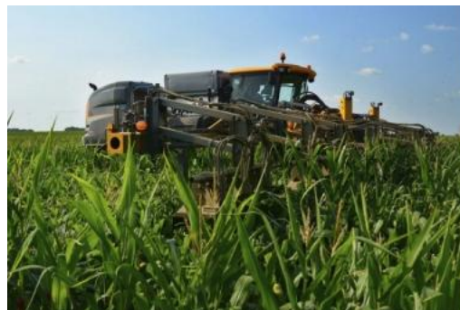
Fig. 15 - Hagie DTB-series corn detasseling machine
