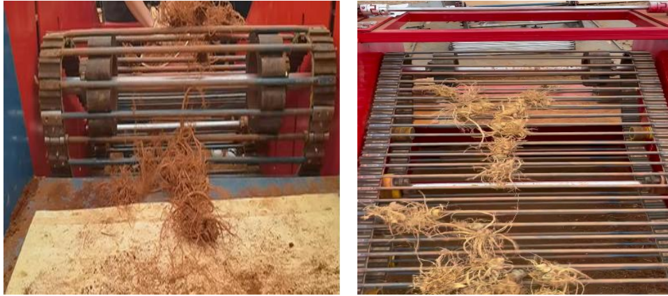
Fig. 23 - Separation conveyor device lab test
