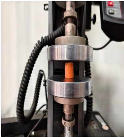
Fig. 5 - Sweet potato samples placed on the testing machine platform
