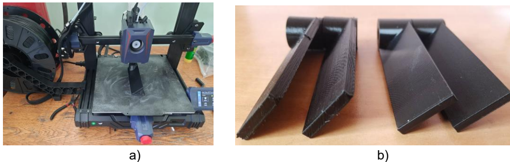
Fig. 3 – Photograph of the blade manufacturing process with an inclination angle of \zeta = 45^\circ by 3D printing (a) and the manufactured blades with inclination angles of \zeta = 40^\circ and \zeta = 50^\circ (b).
