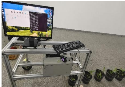
Fig. 4 - Indoor simulated operation platform for edge deployment and virtual spraying signal verification.
