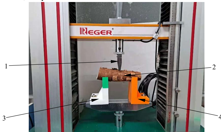
Fig. 4 - Bending test of cassava roots
