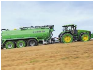
(a) John Deere 8R 410 Hybrid (USA) (Series-Parallel Power-Split Type, 2024)
