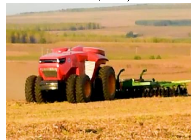
(f) "Honghu" T300 High-Power Hybrid Tractor (400 HP New Energy Intelligent Agricultural Machinery, 2022)
