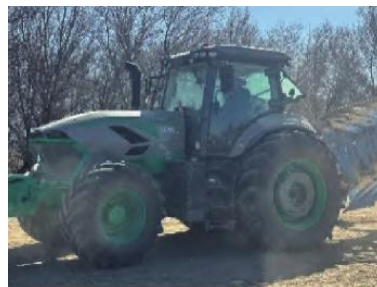
(h) SDLG T3204-7E Tractor (Series-Parallel Power-Split Type, 2024)
