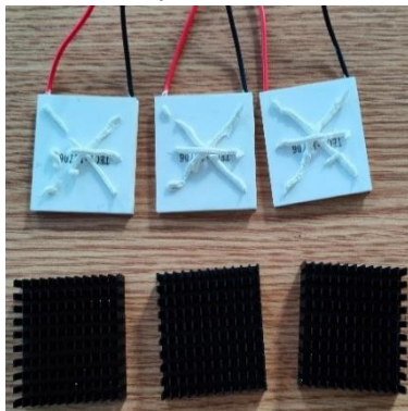
Fig. 8 - Heat-sink mounting using thermal paste
