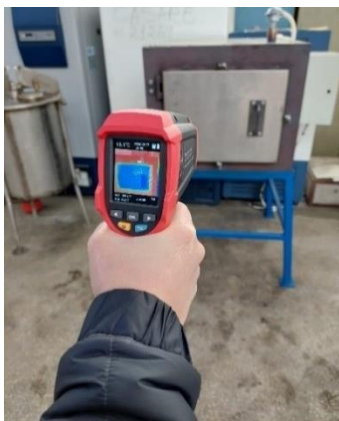
Fig. 14 - Measurement of the equipment surface temperature
