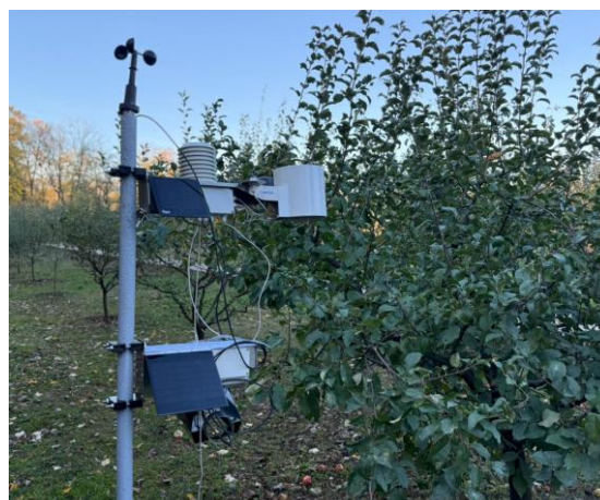
Fig. 6 – Integrated experimental monitoring platform installed under orchard field conditions
