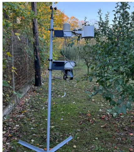
Fig. 2 – Experimental meteorological station used for continuous orchard environmental monitoring
