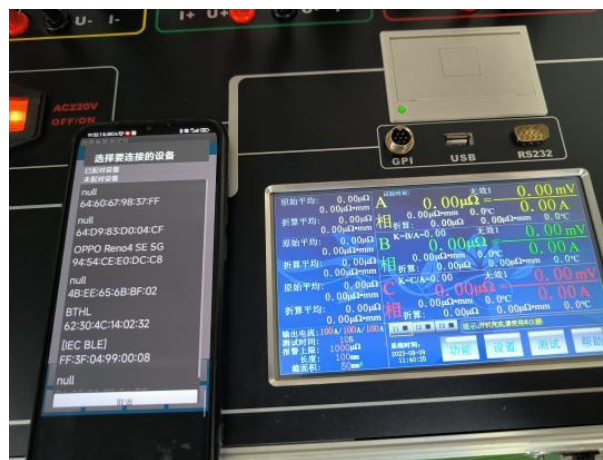
Fig. 15 – Field measurement image of the loop resistance tester
