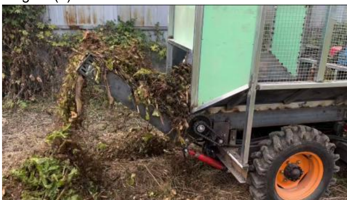
(a) Automatic unloading process of crushed tobacco stems
