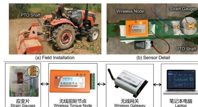
Fig. 1 – Schematic diagram of wireless torque testing system
