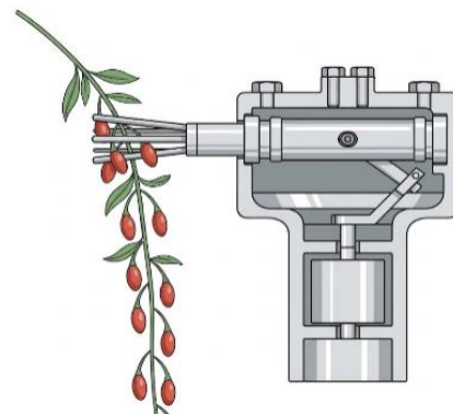
Fig. 7 - Operation Diagram of the Portable Harvesting Device
