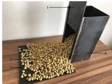
Fig. 5 - Device for measuring the angle of repose of soybean seeds
