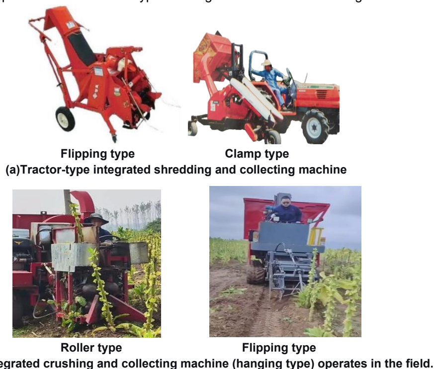
Fig. 4 - Integrated tobacco stalk harvester
