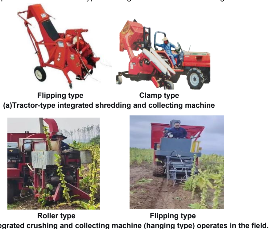
Fig. 4 - Integrated tobacco stalk harvester
