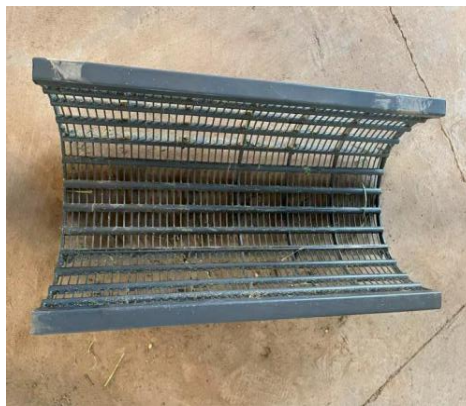
Fig. 4 – Round steel bar concave screen
