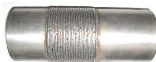
Fig. 2 – Specimen with deposited weld coating
