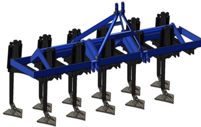
Fig. 1 - Three-dimensional model of the cultivator developed using SolidWorks software
