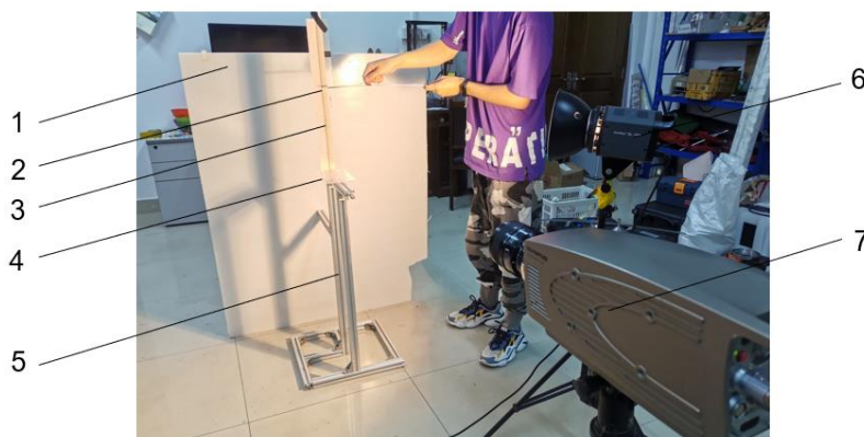
Fig. 4 - High-speed imaging system for restitution coefficient measurement
